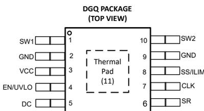
**Figure 4-1. Pin Diagram (DGQ-10) package**
