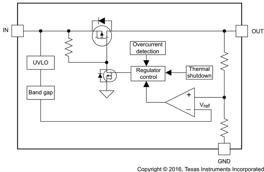
**Figure 1-1. Functional Block Diagram**
