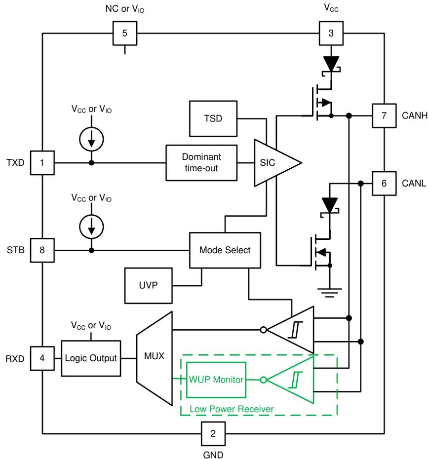
**Figure 1-1. TCAN1462-Q1 and TCAN1462V-Q1 Functional Block Diagram**
