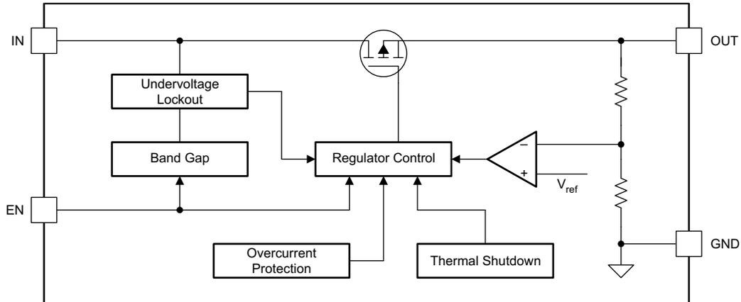
**Figure 1-1. Functional Block Diagram**
