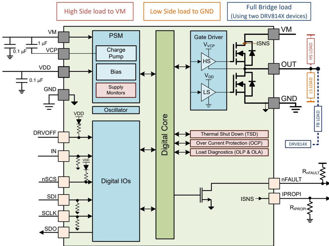
Figure 1-3. Functional Block Diagram for SPI "P" variant
