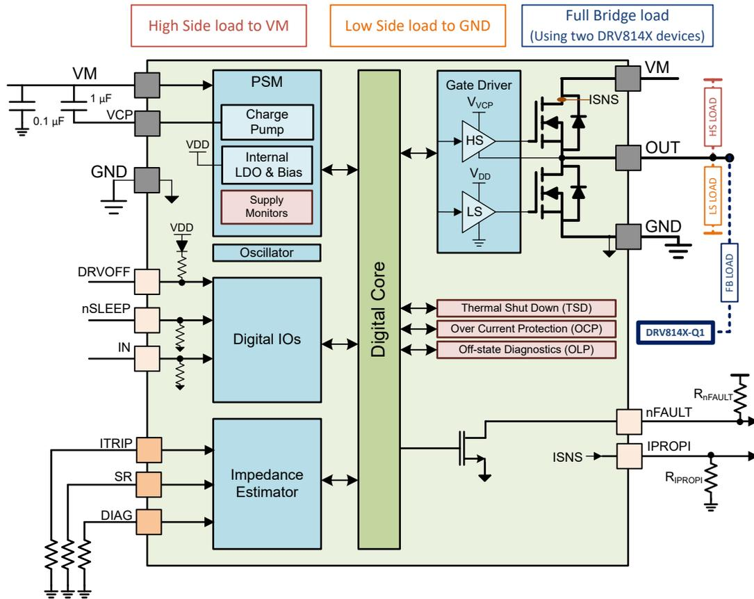
**Figure 1-1. Functional Block Diagram for HW variant**
