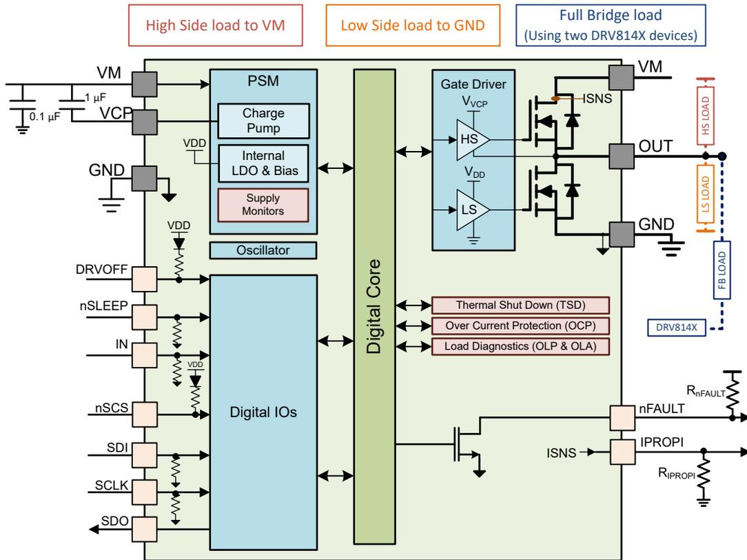
Figure 1-2. Functional Block Diagram for SPI "S" variant
