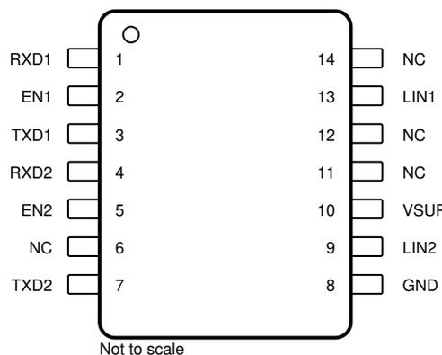
**Figure 4-2. D Pin Diagram**
