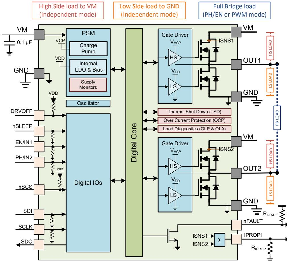
Figure 1-2. Functional Block Diagram for SPI "S" variant
