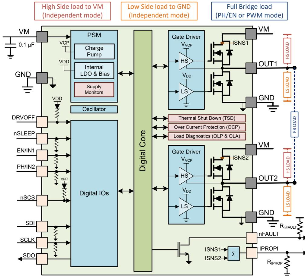
Figure 1-3. Functional Block Diagram for SPI "P" variant
