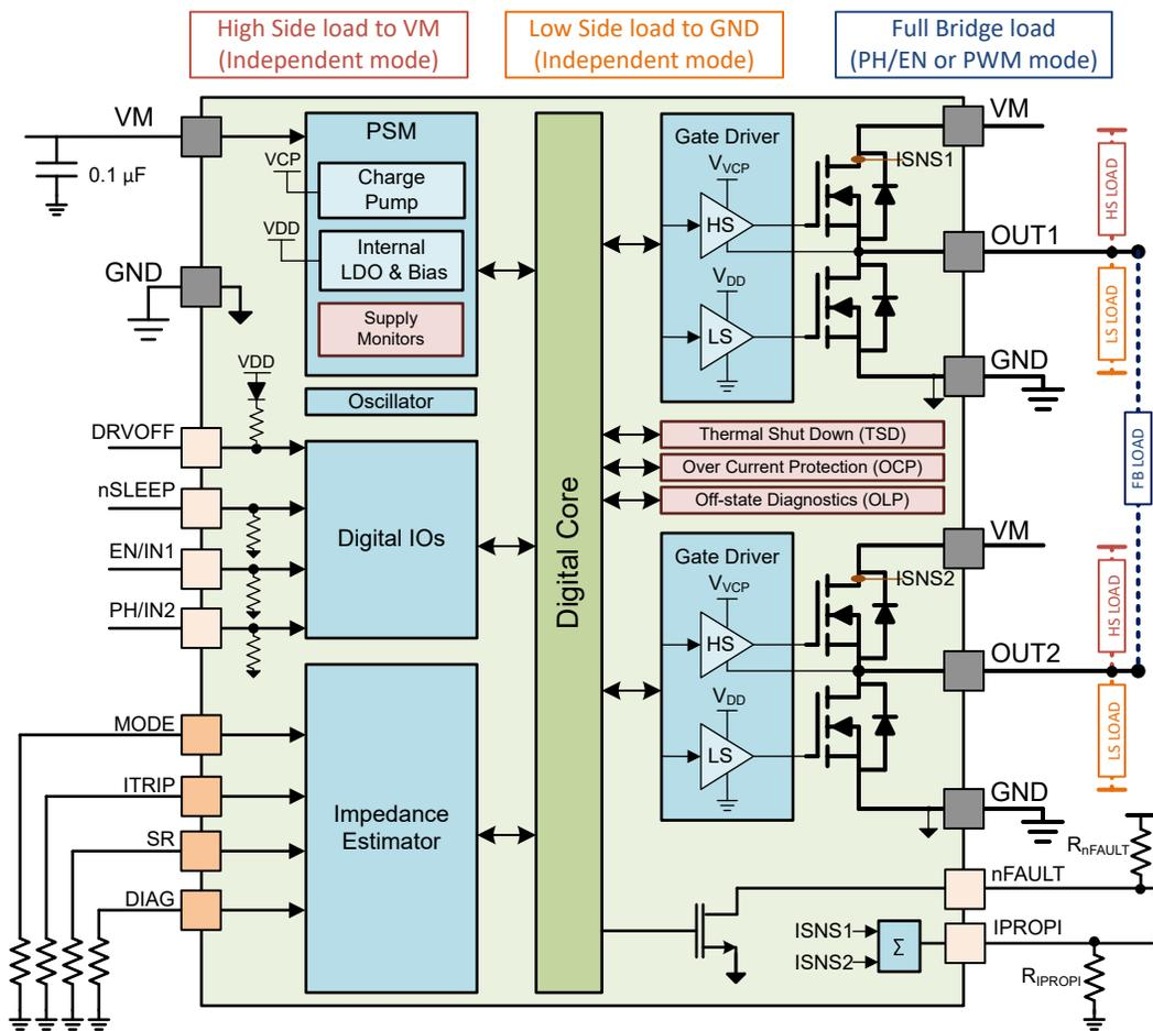
Figure 1-1. Functional Block Diagram for HW variant
