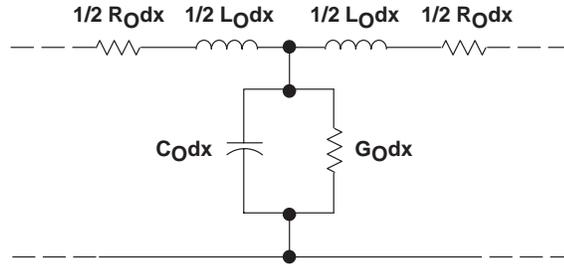
**Figure 9. Transmission-Line Components**
