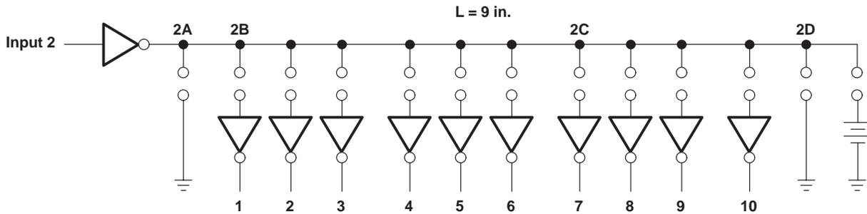
Figure 17. Schematic Diagram of a Distributed Loaded System
