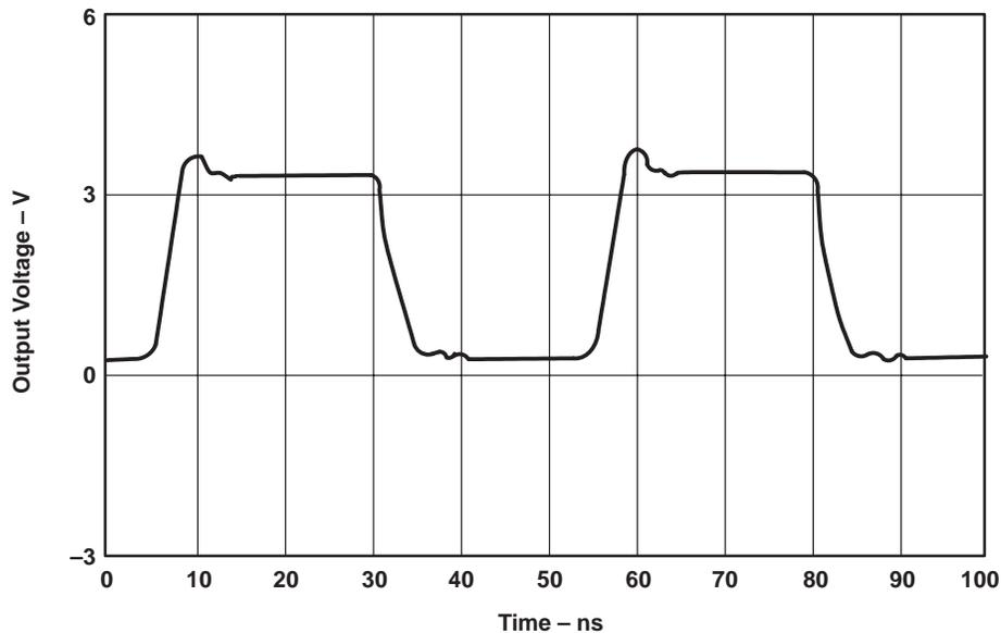
Figure 25. Parallel-Termination Waveform
