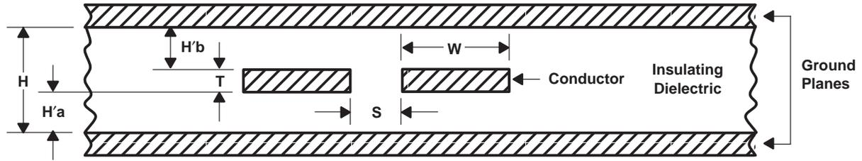
Figure 12. Strip-Line Structure
