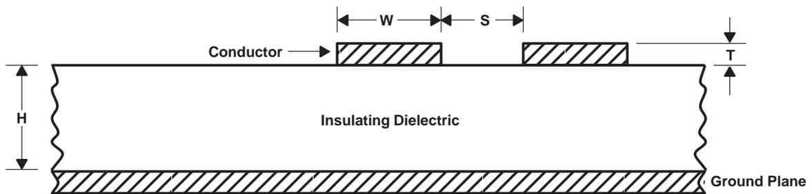
Figure 11. Microstrip-Line Structure
