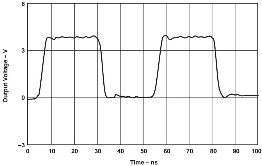
**Figure 28. Series-Termination Waveform**
