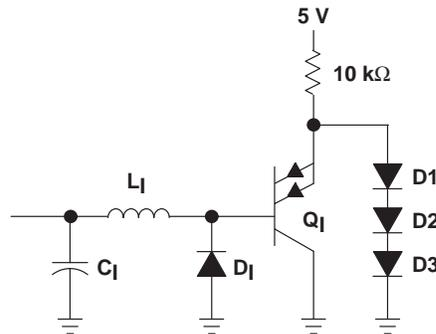
Figure 6. AS Input Structure
