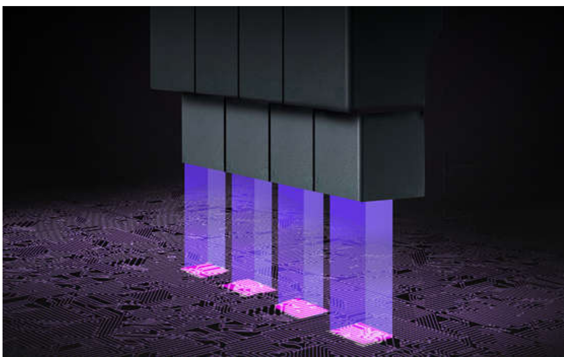
Figure 1. Maskless Photolithography using a DLP DMD
