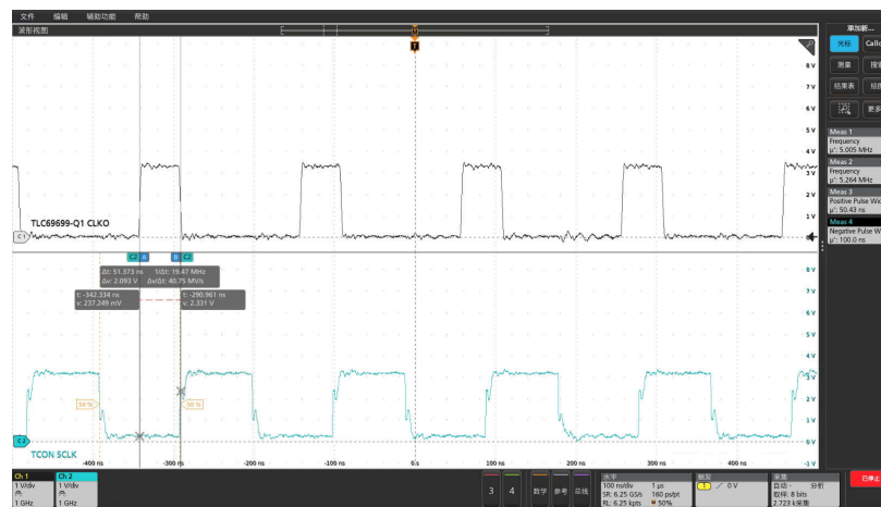
Figure 3-6. TLC69699-Q1 Input and Output Frequency Control with TXFIFO
