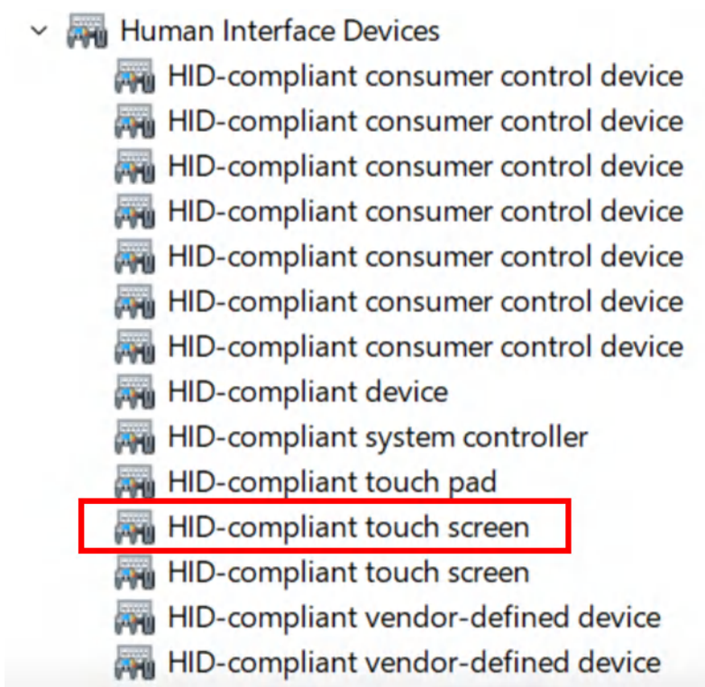
Figure 4-3. PC Device Manager View of USB HID Touch Screen Devices
