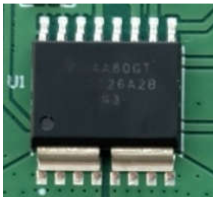
Figure 2-2. SOIC-10 package on SOIC-16 Footprint
