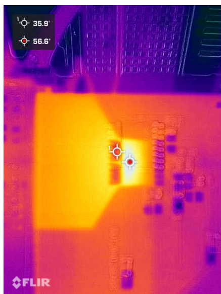
Figure 2-12. SOIC-10 on SOIC-16 Footprint, Post-500 Cycles, SAC Water Soluble Paste
