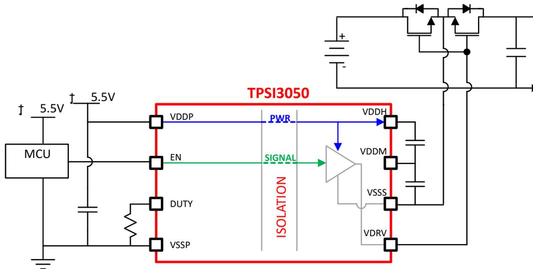
Figure 2-1. TPSI3052 Simplified Schematic
