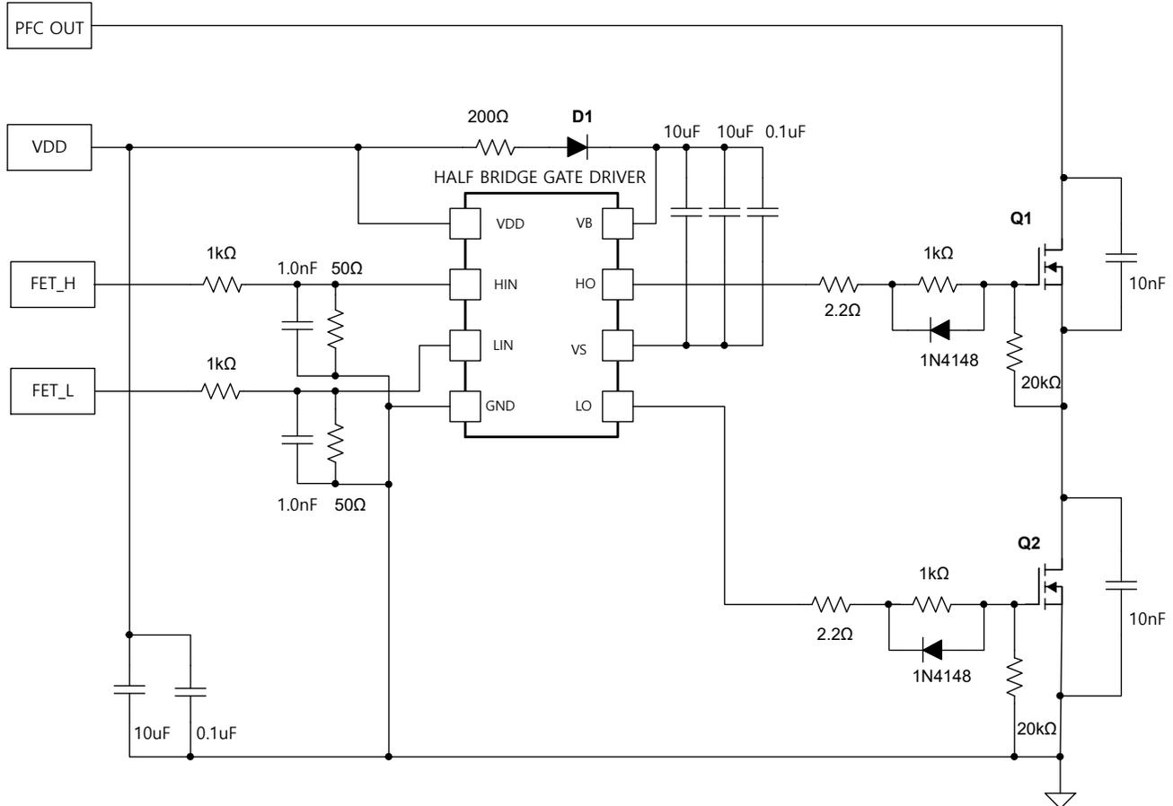
Figure 4-1. Conventional Circuit for Operating PFC Slow Switch at High-side (Q1)
