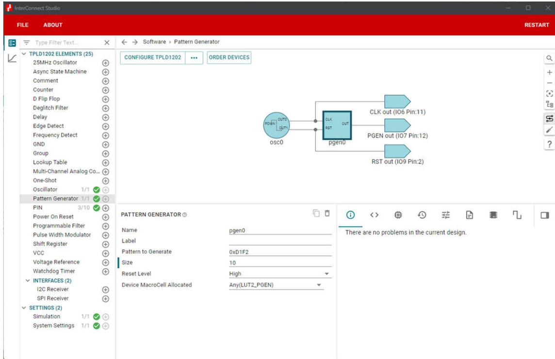
**Figure 3-1. PGEN With Reset (10-bit Pattern, 0x1F2) Example Configuration in ICS**
