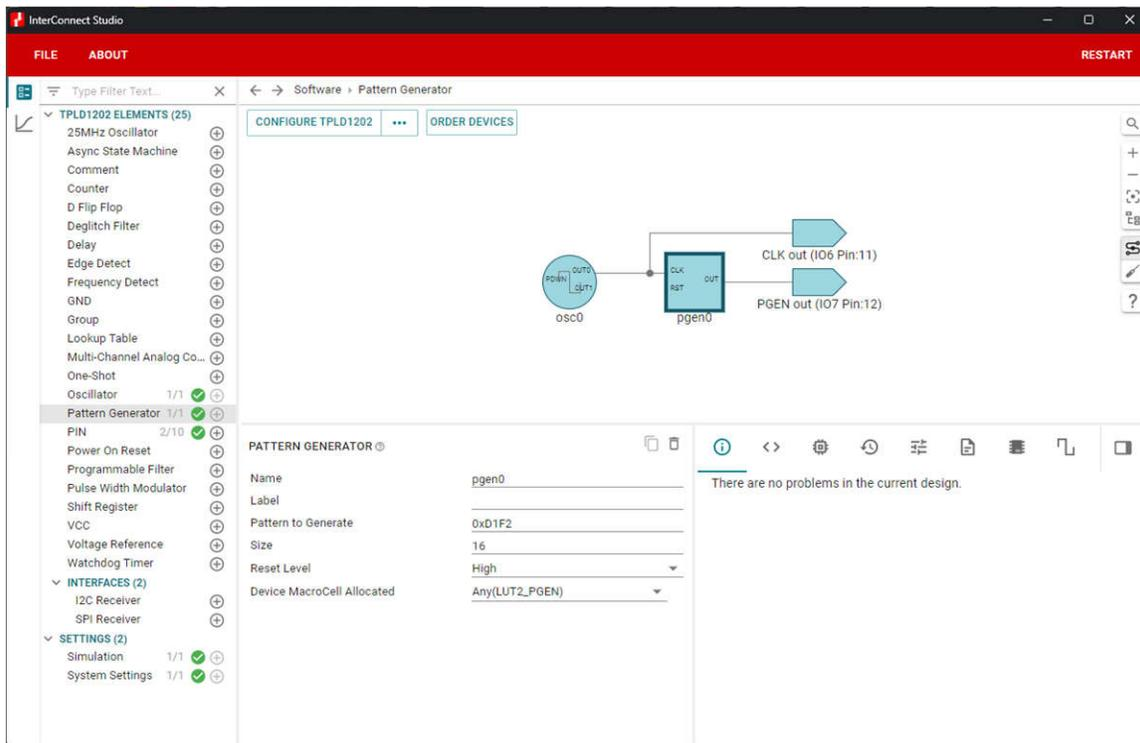
**Figure 1-2. Pattern Generator (PGEN) Configuration in ICS**
