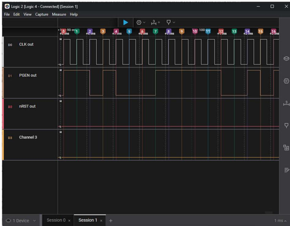
**Figure 1-3. Logic Analyzer Capture of Pattern Generator Output**
