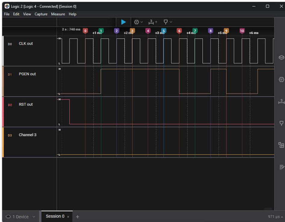
Figure 3-3. Logic Analyzer Capture of PGEN With Reset (10-bit Pattern, 0x1F2, Zoomed)
