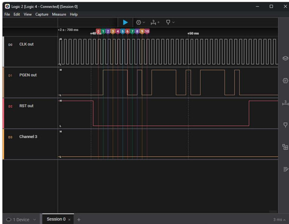
**Figure 3-2. Logic Analyzer Capture of PGEN With Reset (10-bit Pattern, 0x1F2)**
