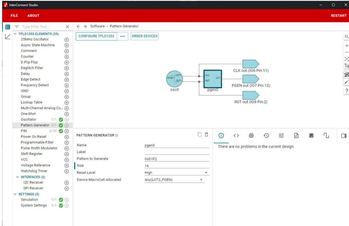
Figure 2-1. PGEN With Reset (16-bit pattern, 0xD1F2) Example Configuration in ICS
