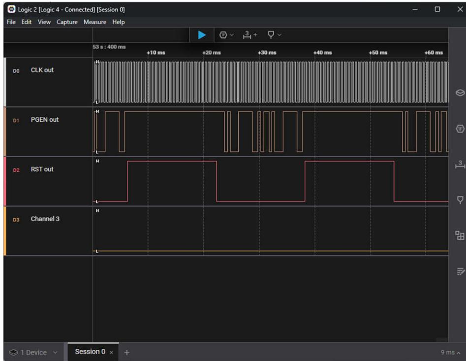
Figure 2-2. Logic Analyzer Capture of PGEN With Reset (16-bit Pattern, 0xD1F2)
