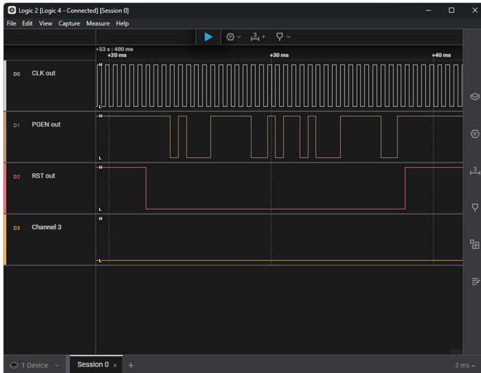
Figure 2-3. Logic Analyzer Capture of PGEN With Reset (16-bit Pattern, 0xD1F2, Zoomed)
