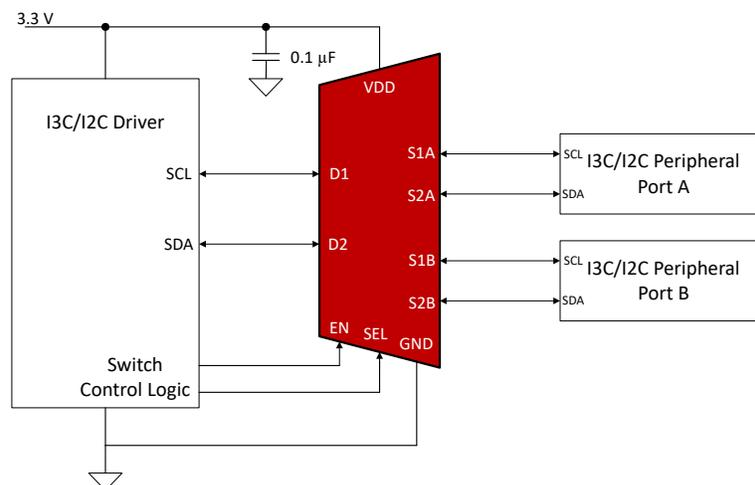
**Figure 4. TMUX121 Typical I3C Application**
