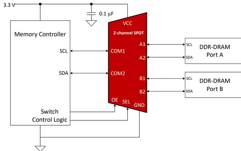
**Figure 3. I3C DDR-DRAM Switch Example**
