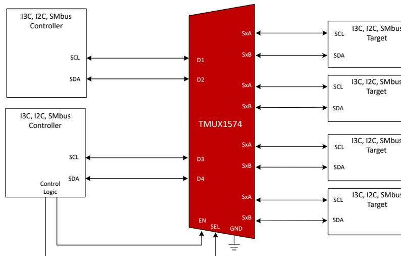
Figure 6. Multiplexing Two I3C Lanes with TMUX1574
