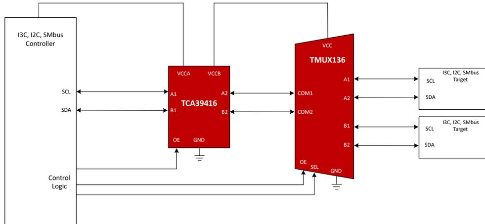
**Figure 7. Flexible 2:1 I3C Bus with Signal Boost - TMUX136 + TCA39416**
