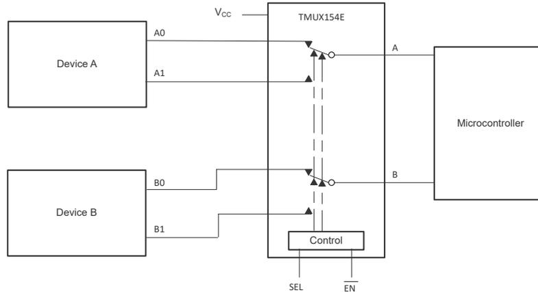
Figure 5. TMUX154E Application Diagram
