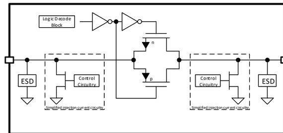
**Figure 2-1. Current Injection Control Circuitry**
