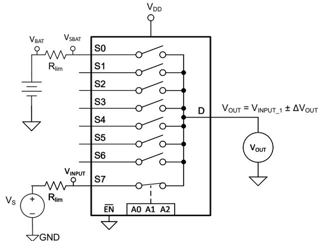
**Figure 2-2. Channel S7 Selected, Channel S0 Experiencing a Short-to-Battery Condition**
