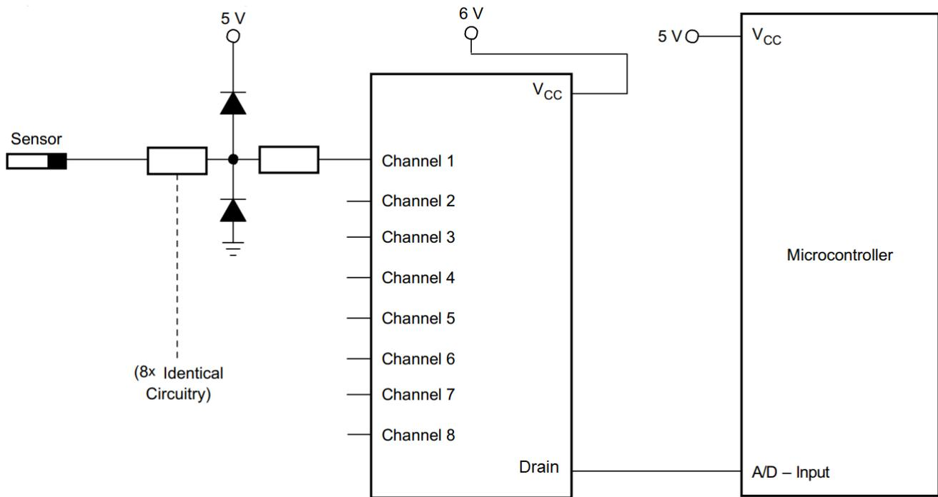
Figure 1-1. External Passive Components Implementation
