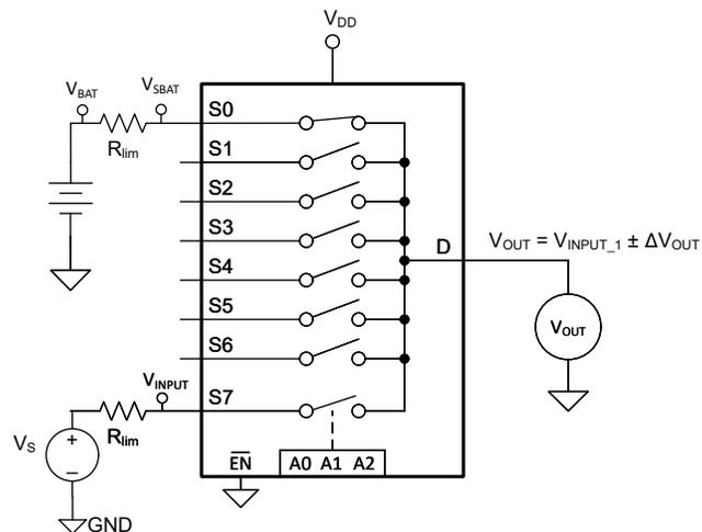
Figure 2-4. Short-to-Battery Condition Only on a Single Selected Channel
