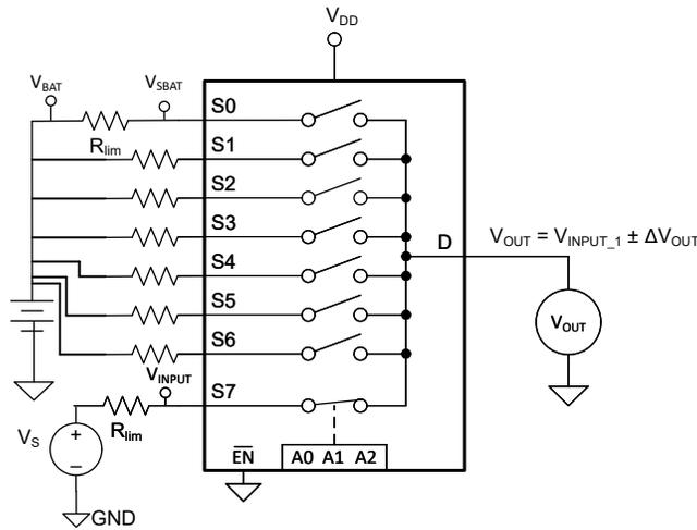
Figure 2-3. All Unselected Channels Experiencing a Short-to-Battery Condition
