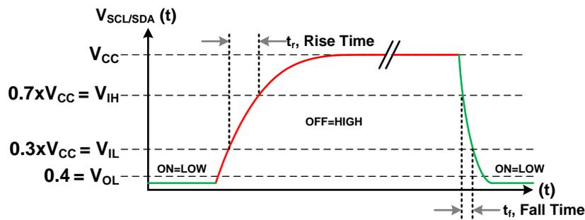
Figure 5. I<sup>2</sup>C Waveform with Logic Level, Rise Time, and Fall Time Information for SCL and SDA
