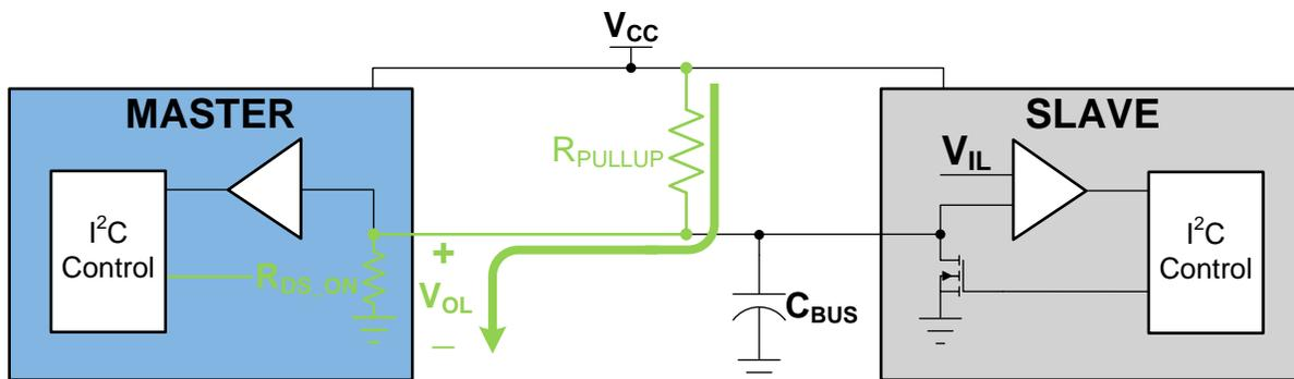
Figure 6. Resistor Divider Created when Pull Down FET is on With the Pullup Resistor and How V<sub>OL</sub> is Determined
