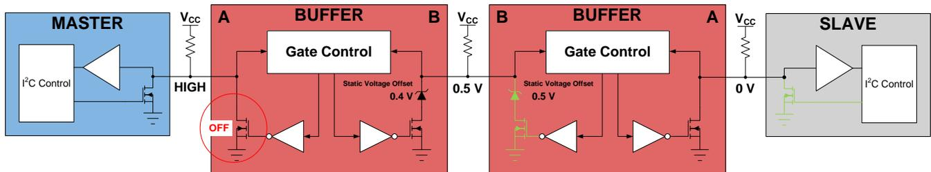
Figure 19. Diagram for Propagating a Low from the Slave to the Master Which Shows the Master Failing to see the Low.
