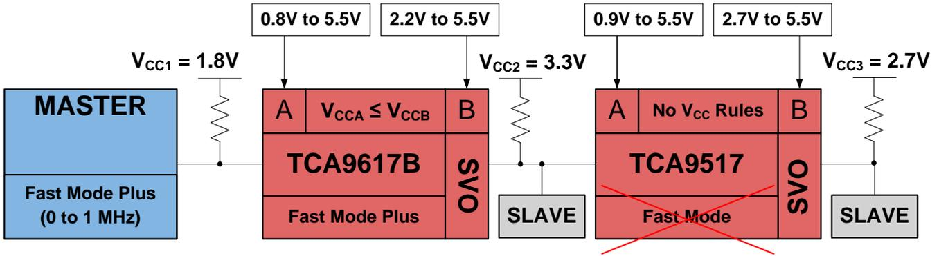
Figure 23. TCA9517 Does not Support Fast Mode Plus
