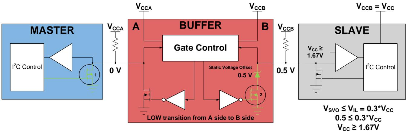
Figure 15. Diagram of how to Check of the SVO is not Violating the V<sub>IL</sub> of the Slave Device
