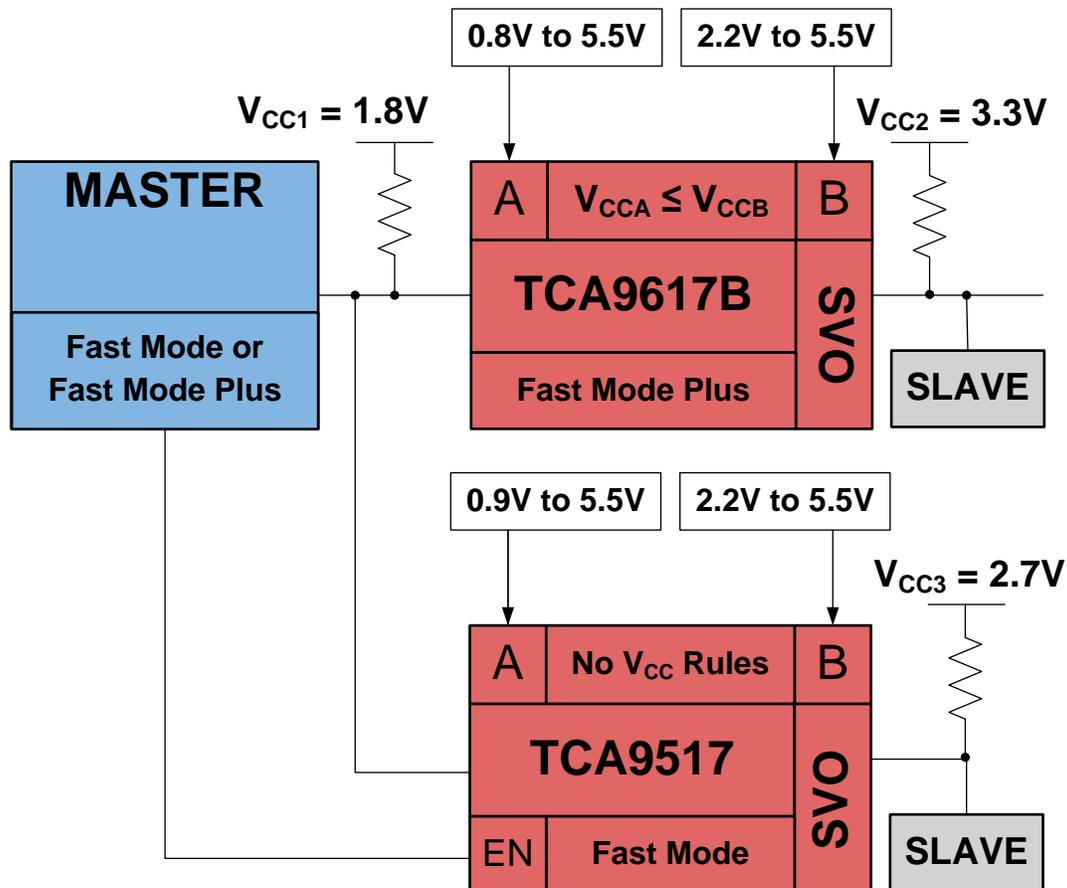
Figure 25. Example of an I<sup>2</sup>C System with Two Slaves that Operate with Two Modes of Operation
