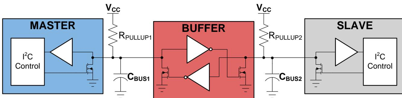
Figure 7. How C<sub>BUS</sub> and R<sub>PULLUP</sub> gets Subdivided into C<sub>BUS1</sub>, R<sub>PULLUP1</sub>, C<sub>BUS2</sub>, and R<sub>PULLUP2</sub> Using a Buffer
