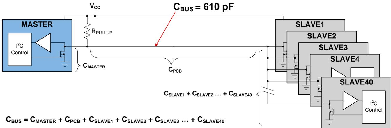
**Figure 8. Example I<sup>2</sup>C System that Includes Capacitance on the Bus due to Master, PCB, and all the Slaves on the Bus**
