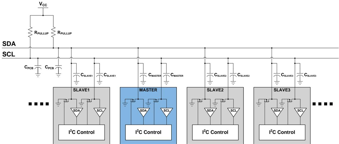
$$C_{BUS} = C_{PCB} + C_{MASTER} + C_{SLAVE1} + C_{SLAVE2} + C_{SLAVE3} + \dots$$
