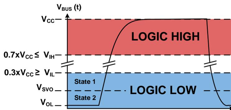
Figure 11. Diagram of Valid Logic High and Logic Low Levels for I<sup>2</sup>C and the Two States Created with a Static Voltage Offset.
