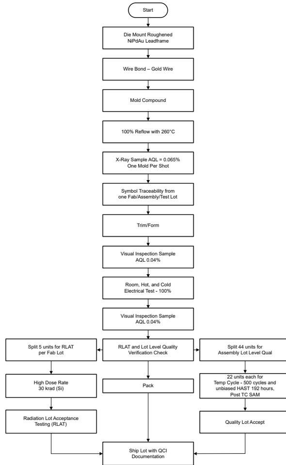
Figure 2-1. SN54SC6T17-SEP Space Enhanced Plastic Production Flow Chart
