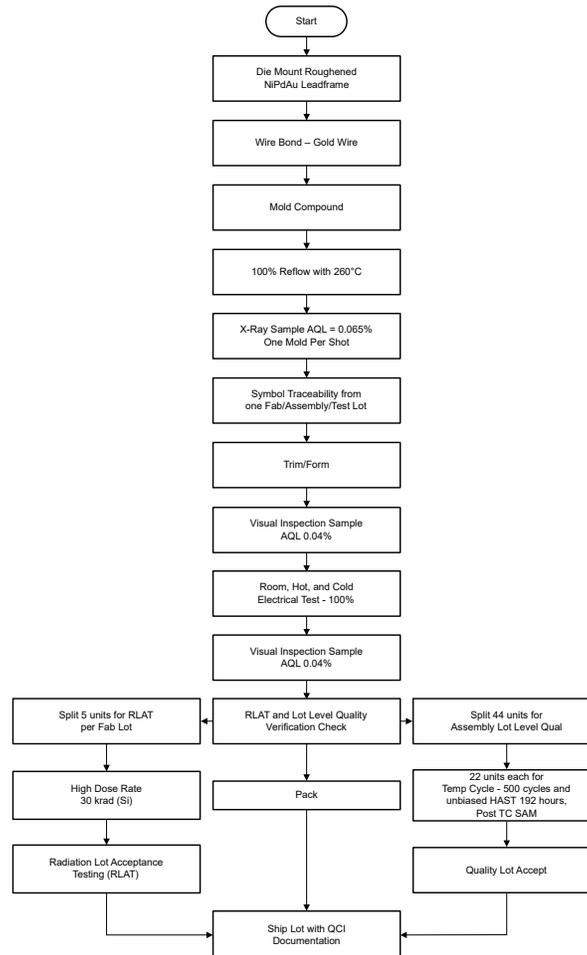
**Figure 2-1. SN54SC6T14-SEP Space Enhanced Plastic Production Flow Chart**
