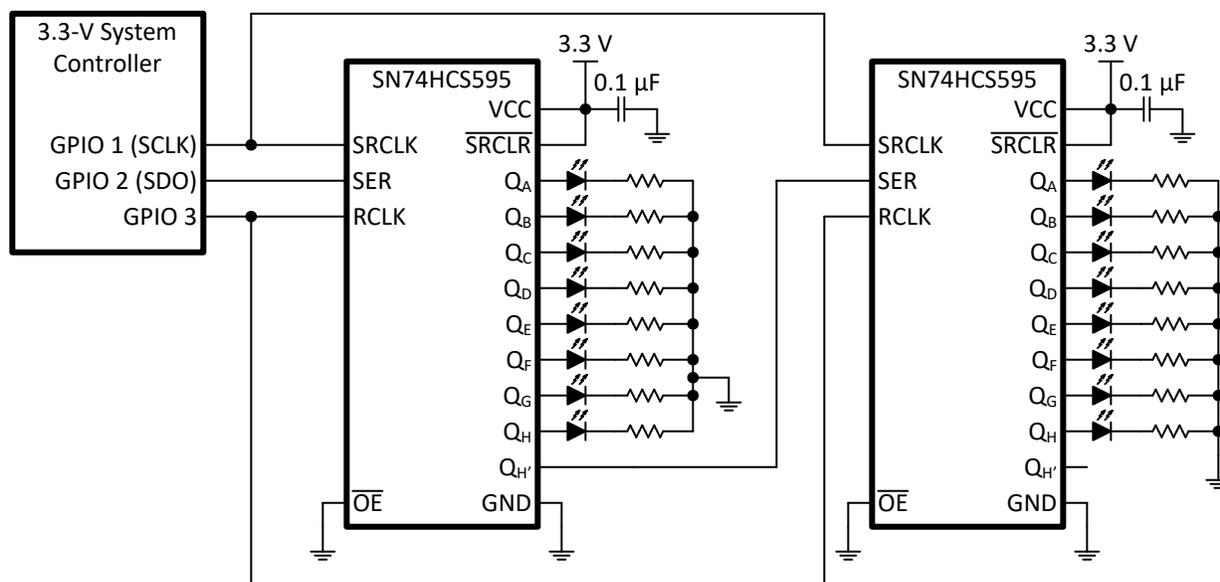
**Figure 2. Example Schematic of Driving 16 Indicator LEDs with Shift Registers Using Only 3 Control Pins**
