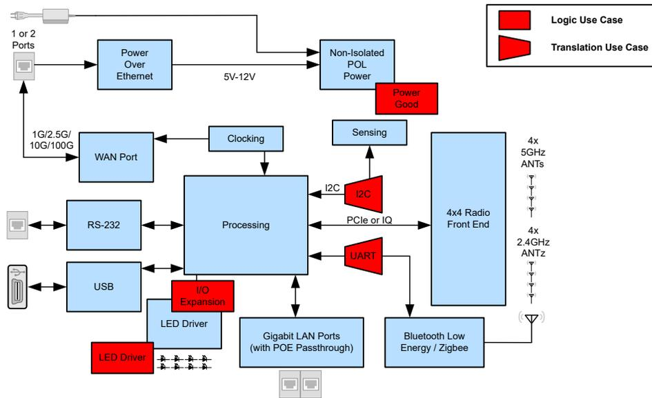
Figure 1. Simplified Block Diagram for WLAN and Wi-Fi Access Points
