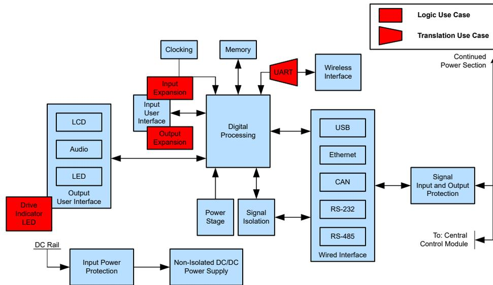
**Figure 2. Simplified Block Diagram for DC Fast Chargers Human-Machine Interface Section**
