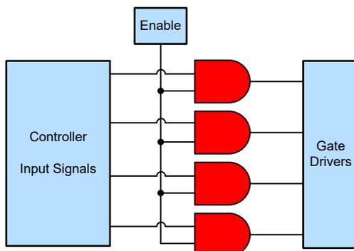
**Figure 3. Example block diagram to use AND gates to enable gate driver signals**
