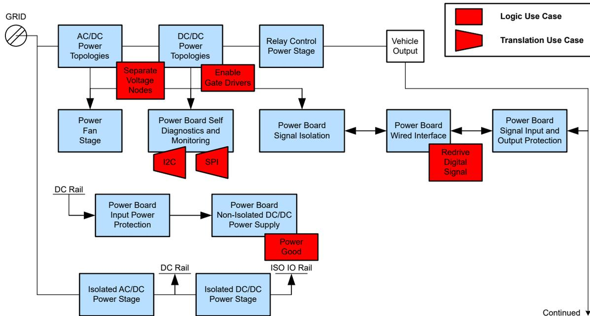
Figure 1. Simplified Block Diagram for DC Fast Chargers Power Section
