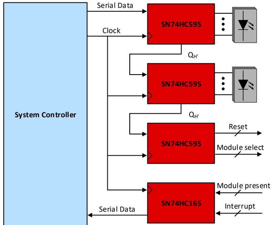
**Figure 2-1. I/O Expansion for Network Switch Optical Interface**
