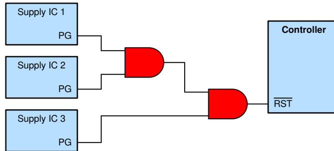
**Figure 3-1. Using Logic to Combine Multiple Power-Good Signals**
