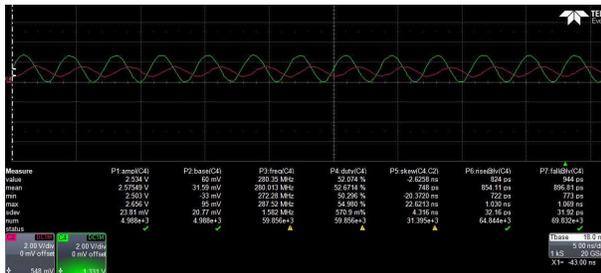
Figure 3-9. TXV Waveform (15 pF 1.8 V to 3.3 V Up Translation at 280 MHz, 25°C)
