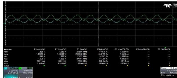
Figure 3-10. Competitor Waveform (15 pF 1.8 V to 3.3 V Up Translation at 280 MHz, 25°C)
