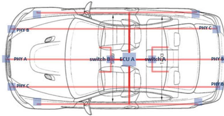
**Figure 1-1. Automotive Example for Data Over Ethernet Using RGMII**
