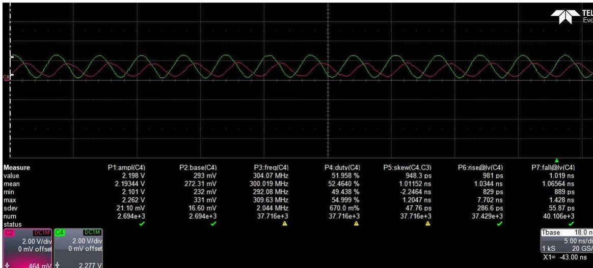
Figure 3-11. TXV Outputs (15 pF 1.8 V to 3.6 V Up Translation at 300 MHz, 25°C)
