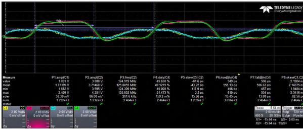
Figure 3-3. TXV Waveform (5 pF 1.8 V to 3.3 V Up Translation at 125 MHz, 125°C)
