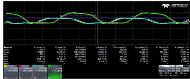
Figure 3-4. Competitor Waveform (5 pF 1.8 V to 3.3 V Up Translation at 125 MHz, 125°C)
