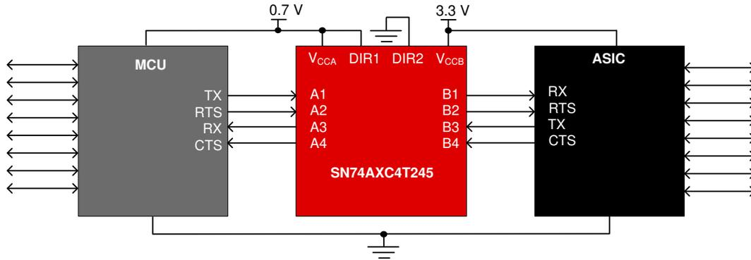
Figure 2-6. 4-wire UART Voltage Translation Using SN74AXC4T245
