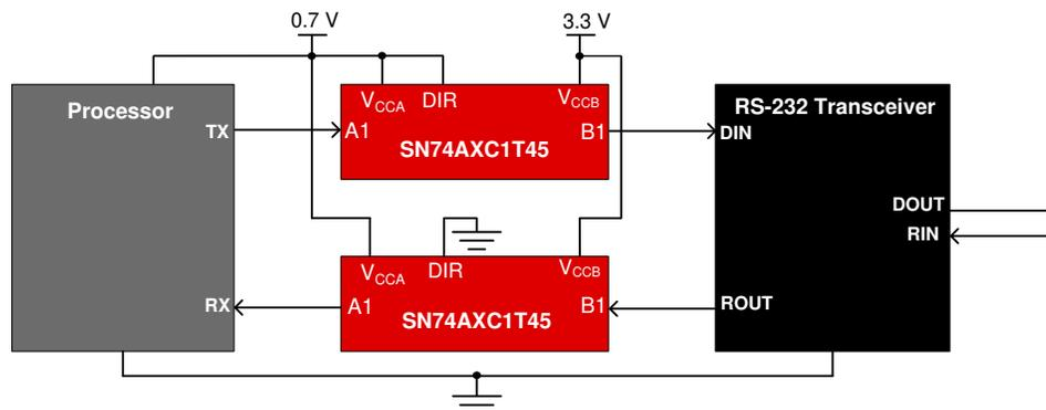
For a simple two line interface, two SN74AXC1T45 on each data line can be implemented to achieve voltage translation. This configuration requires the direction pin on one device to be pulled to  $V_{CCA}$  high to achieve A to B translation, and the DIR pin of the other device pulled to ground to achieve B to A translation as shown in Figure 2-5.
