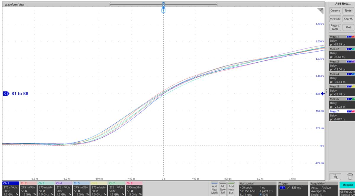
Figure 2-14. 104 ps Channel-to-Channel Skew for SN74AXC8T245
