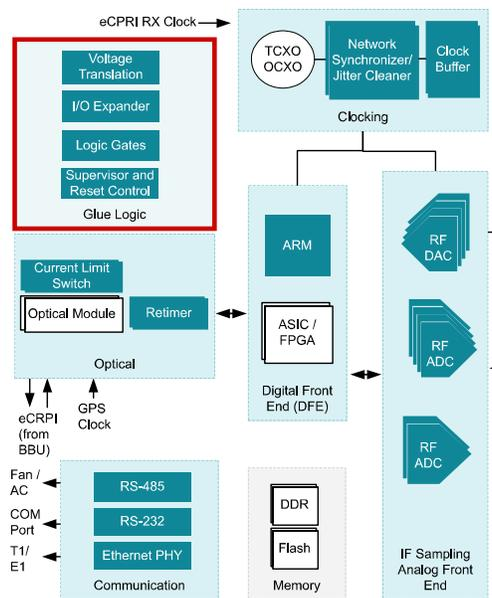
Figure 2-9. UART in Remote Radio Unit
