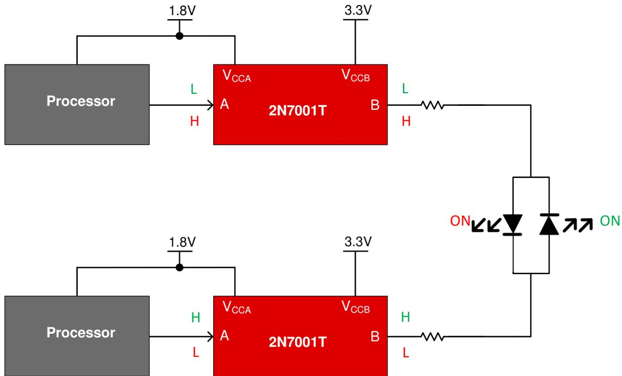
Figure 2-1. Driving LED with Translation Using 2N7001T
