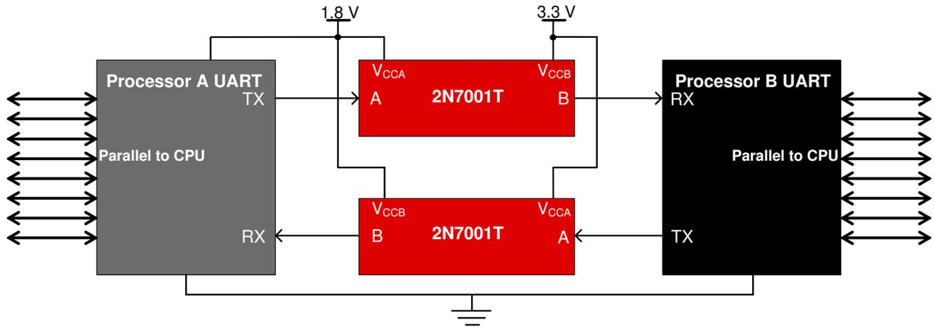
Figure 4-1. Two-Wire UART Interface Using 2N7001T Device
