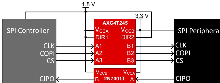
Figure 3-1. SPI Interface Using SN74AXC4T245 and 2N7001T Devices
