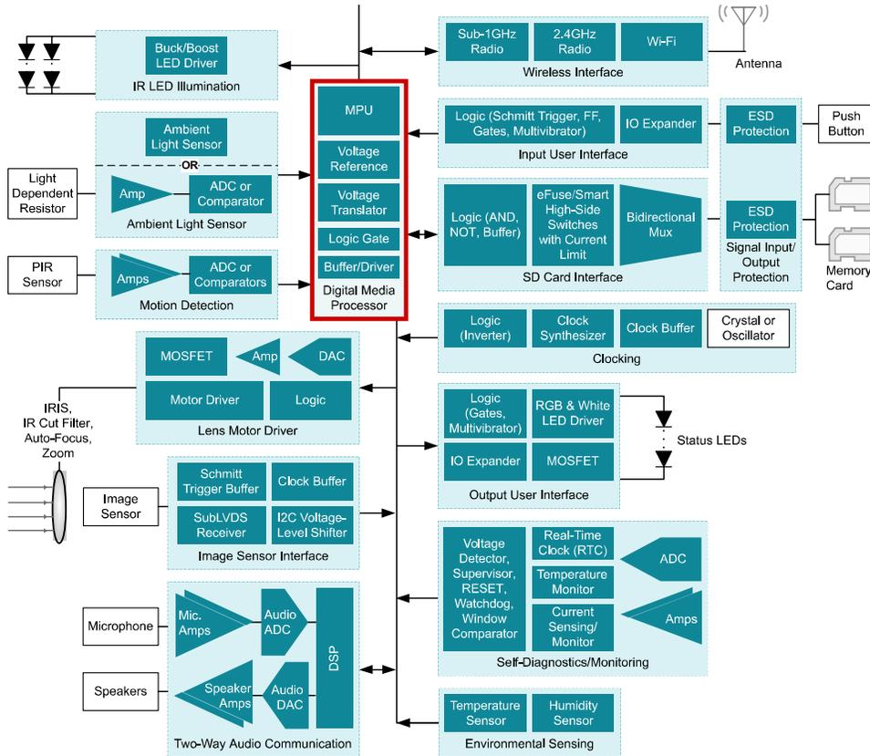
Figure 3-2. SPI Interface in Video Doorbell
