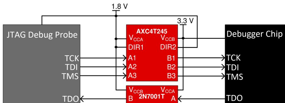
**Figure 5-1. JTAG Interface Using 2N7001T Device**
