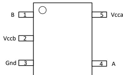
**Figure 1-1. 2N7001T DCK (SC-70) Package**
