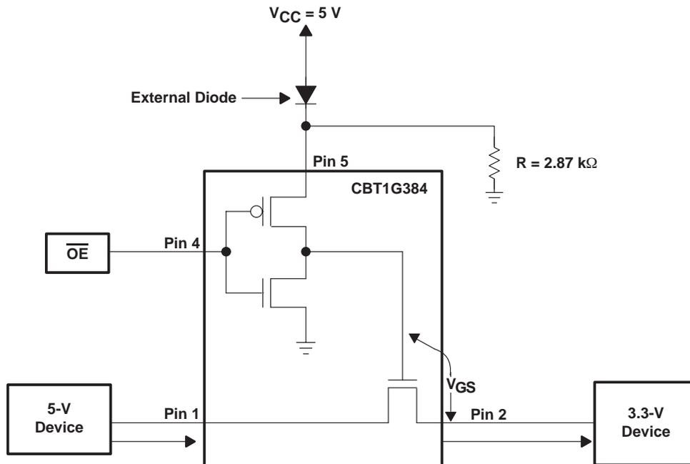
Figure 10. SN74CBT1G384 In 5-V to 3.3-V Application
