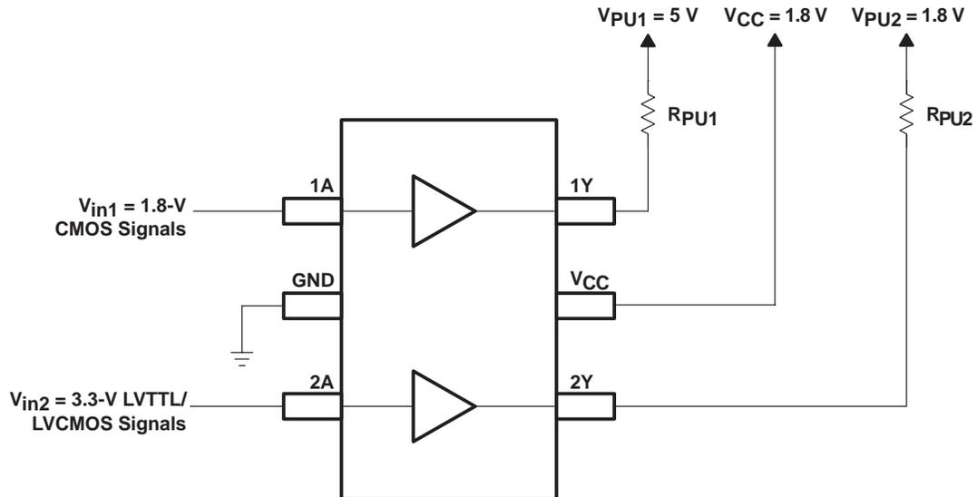
**Figure 6. Use of an Open-Drain Device in a Level-Translation Application**
