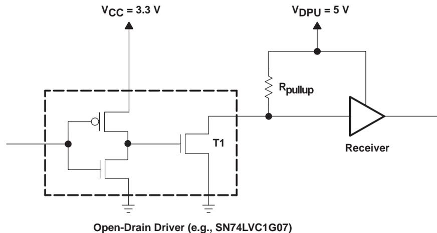
**Figure 5. Level Translation Using an Open-Drain Device**
