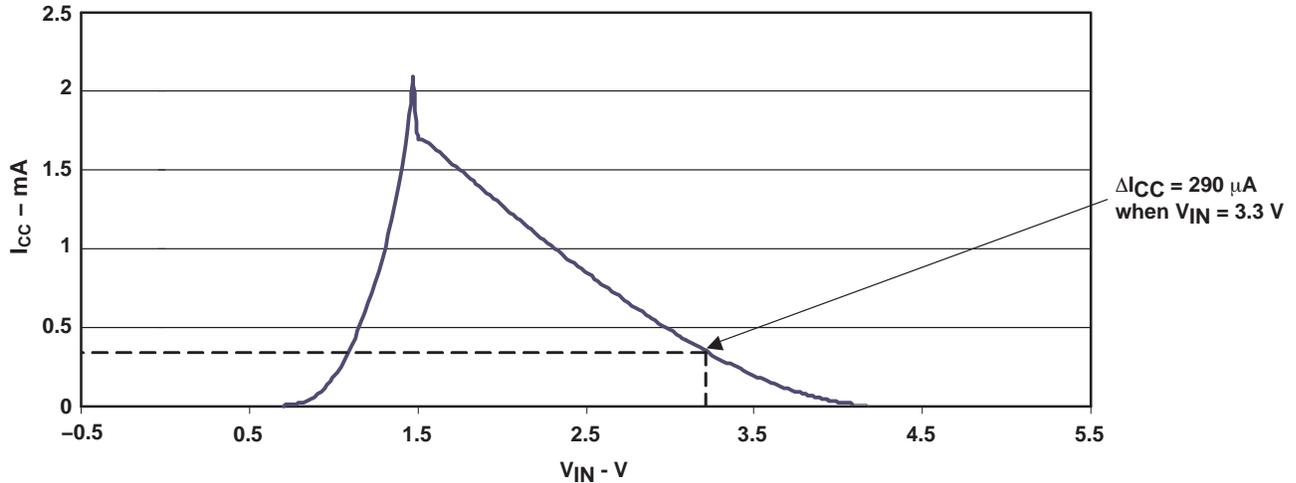
Figure 17.  $V_{IN}$  vs  $I_{CC}$  Characteristics of SN74HCT541
