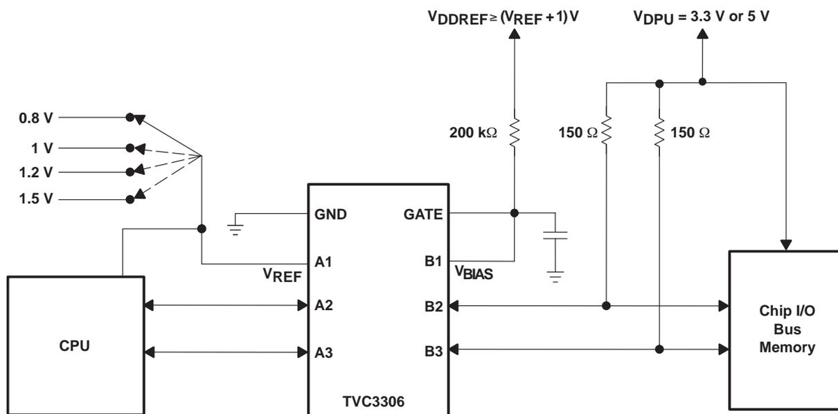
Figure 13. SN74TVC3306 Used in a Level-Translation Application
