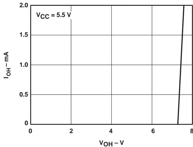
**Figure 4.  $I_{OH}$  vs  $V_{OH}$  for the LVC07A at  $V_{CC} = 5.5$  V**
