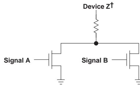
† Open-drain structures of the LVC07A are connected together to provide either an active-high wired-AND or an active-low wired-OR function, depending on signal-A and signal-B levels.
