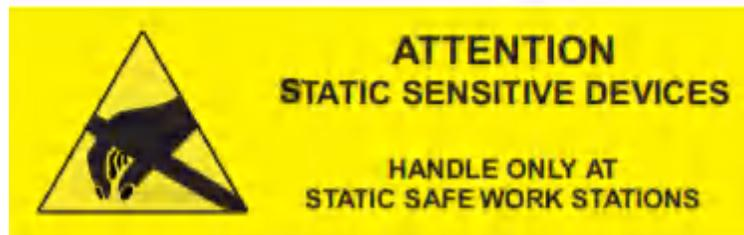
This EVM contains components that can potentially be damaged by electrostatic discharge. Always transport and store the EVM in its supplied ESD bag when not in use. Handle using an antistatic wristband. Operate on an antistatic work surface. For more information on proper handling, see [Electrostatic Discharge \(ESD\)](#).
