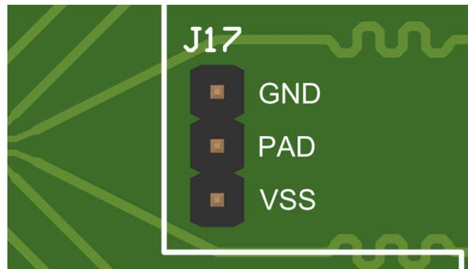
**Figure 5-3. Thermal Pad Selector**
