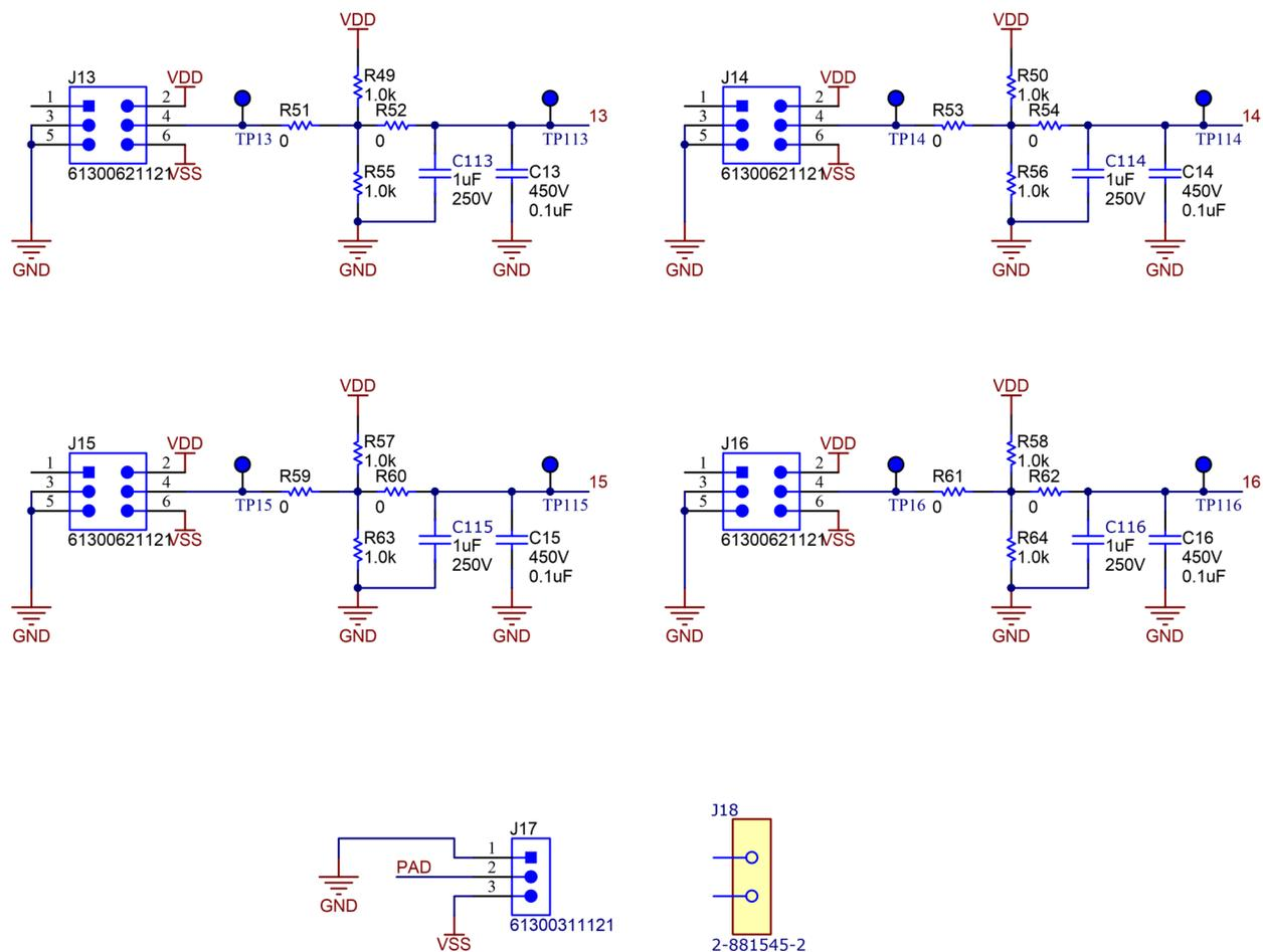
In assembly, connect J18 between pins 1 and 2 of J17.
