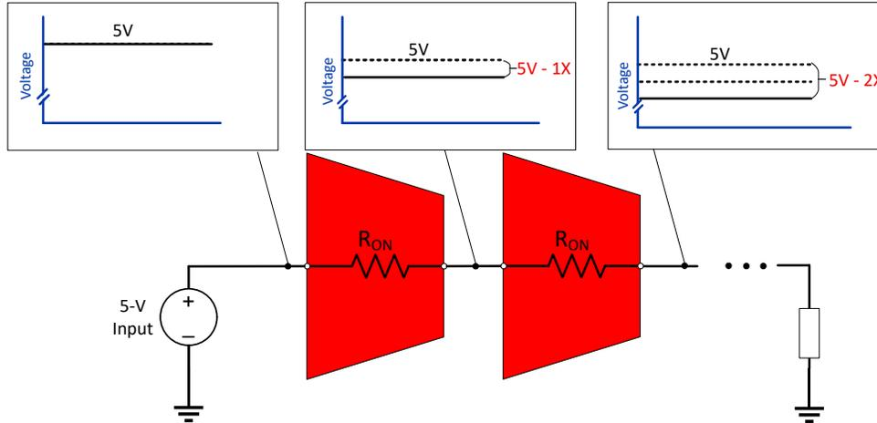
Figure 2-1. Effects of On-Resistance when Cascading Multiplexers
