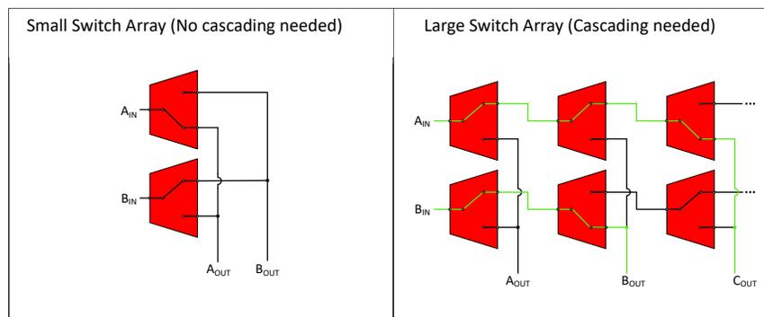
**Figure 1-2. Creating Switch Arrays With Multiplexers**
