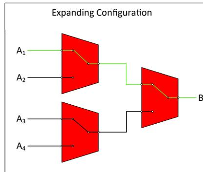
**Figure 1-1. Expanding Configuration With Cascading Multiplexers**
