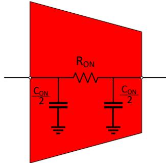
Figure 2-5. Simplified Multiplexer Model
