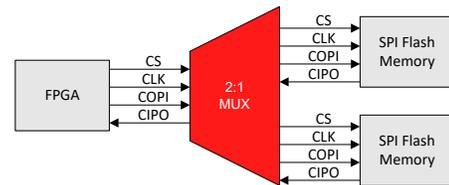
Figure 2. FPGA Access to Multiple Flash Memories
