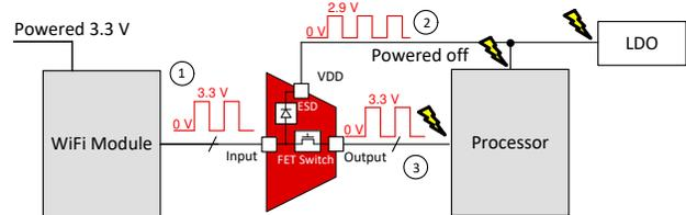
**Figure 1. Subsystem A Back-Powering the Switch**
