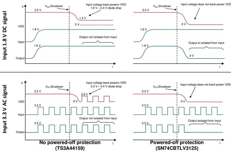
**Figure 3. Signal Switch With and Without Powered-Off Protection**
