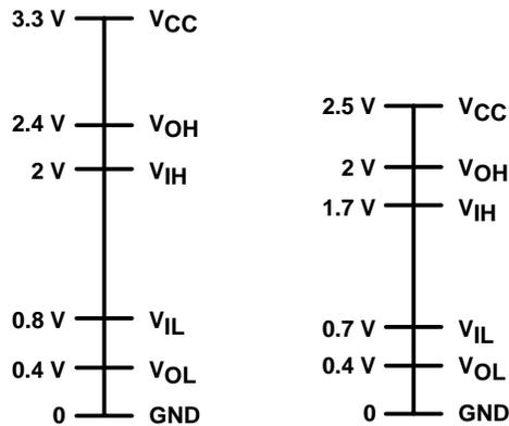
Figure 1. 3.3-V and 2.5-V V<sub>CC</sub> Thresholds
