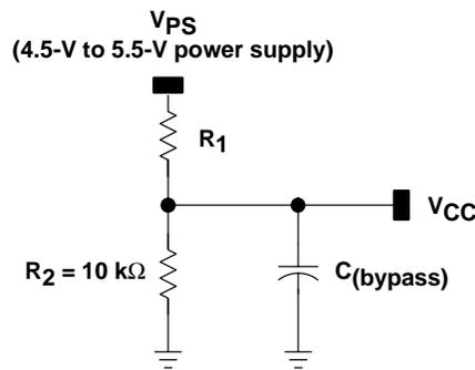
Note:  $C_{(bypass)} = 0.1$  to  $0.01\ \mu\text{F}$
