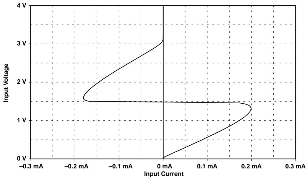
**Figure 17. Bus-Hold Characteristics at LVTTL Input of SN74GTLPH1655**
