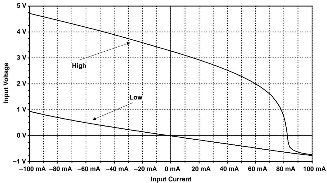
Figure 20. Output Characteristics of LVTTTL Side of SN74GTLPH1655
