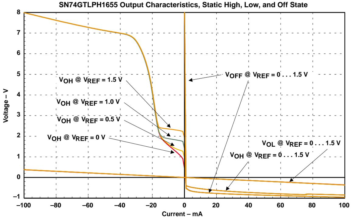
Figure 19. Output Characteristics of GTLP Port of SN74GTLPH1655
