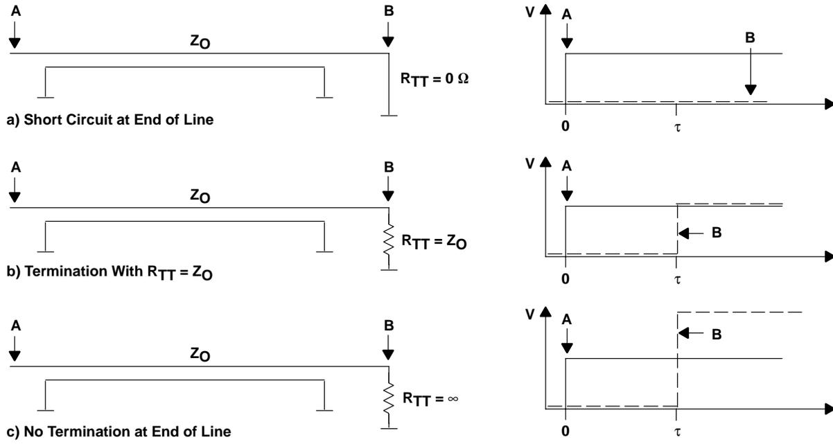
Figure 5. Signals at End of the Line
