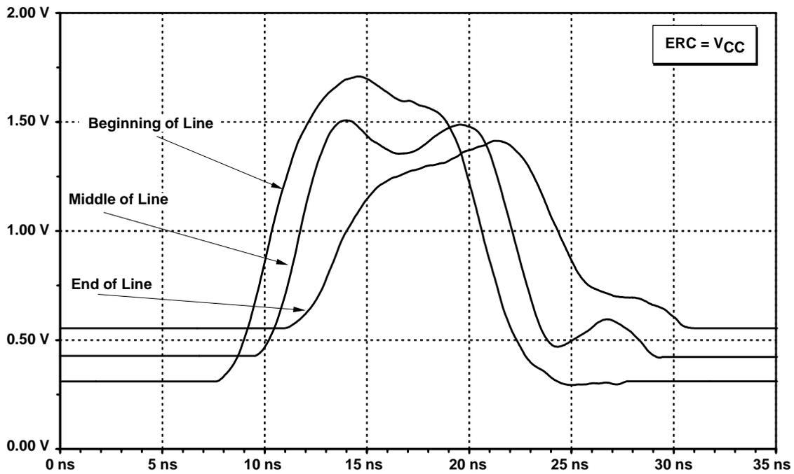
Figure 34. GTP Bus Signal, Slow Rise and Fall Times, ERC =  $V_{CC}$ , Unloaded, 50 MHz
