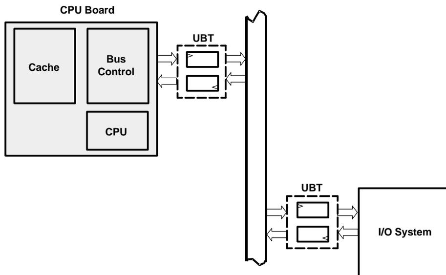
**Figure 12. Typical Bus Application for a UBT**
