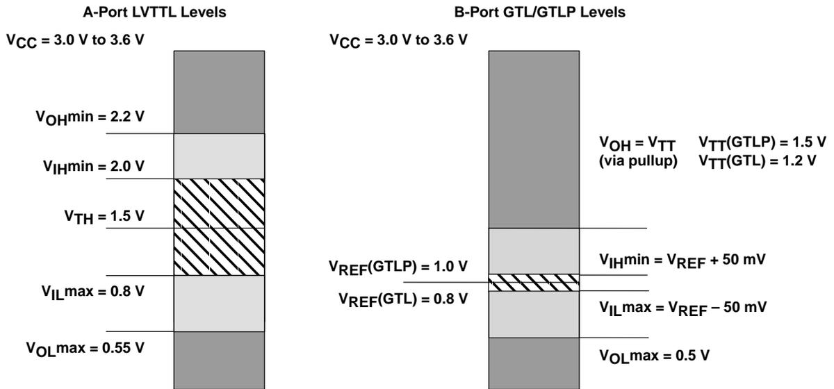
Figure 13. LVTTL and GTLP Signal Levels of SN74GTLPH1655
