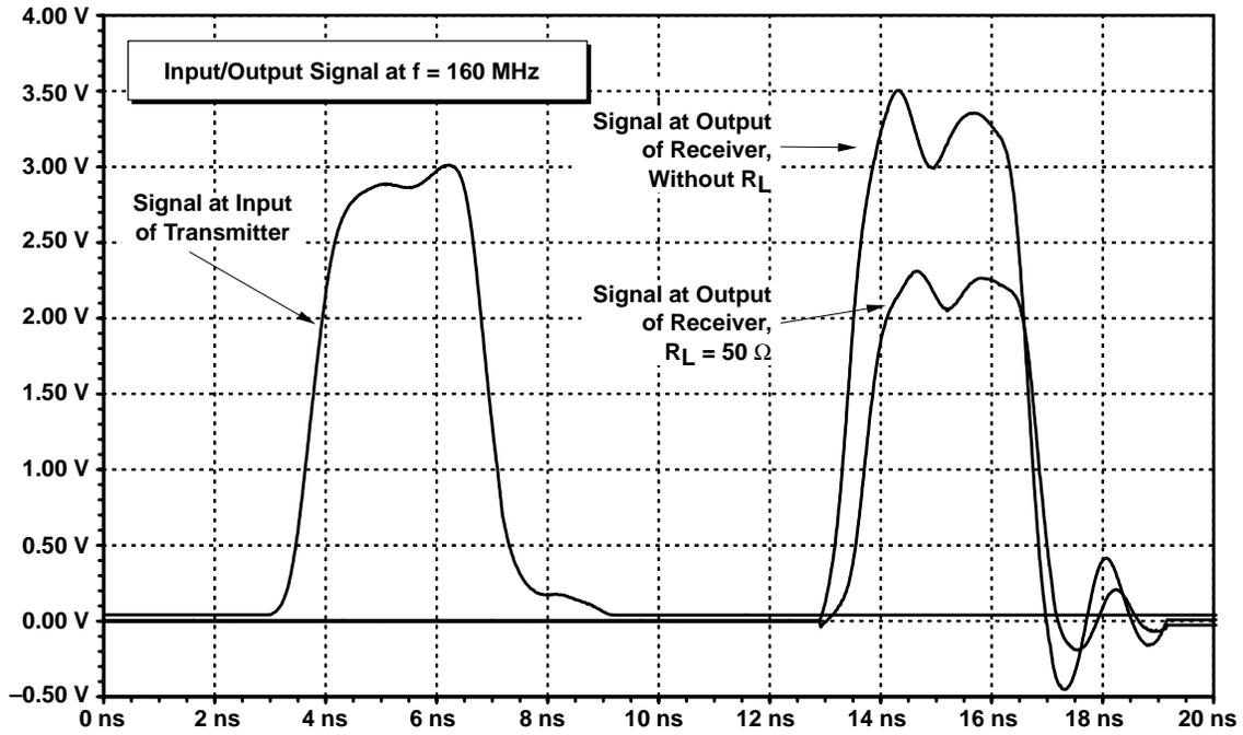
Figure 49. LVTTL Input and Output Signal of SN74GTLPH1655, ERC = V<sub>CC</sub>, Loaded, 160 MHz
