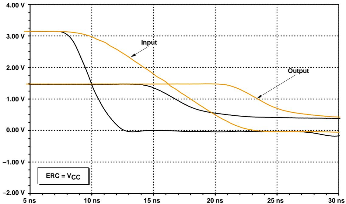
**Figure 23. Falling Edge, ERC = V<sub>CC</sub> (Slow Edges), Input Signals t<sub>f</sub> = 2 ns, 10 ns**
