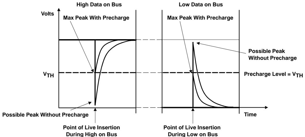
**Figure 27. Influence of Precharge Function on Bus Signal**
