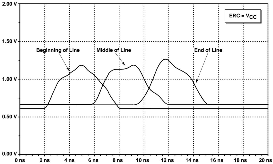
Figure 50. GTLP Bus Signal, Slow Rise and Fall Times, ERC = V<sub>CC</sub>, Loaded, 160 MHz
