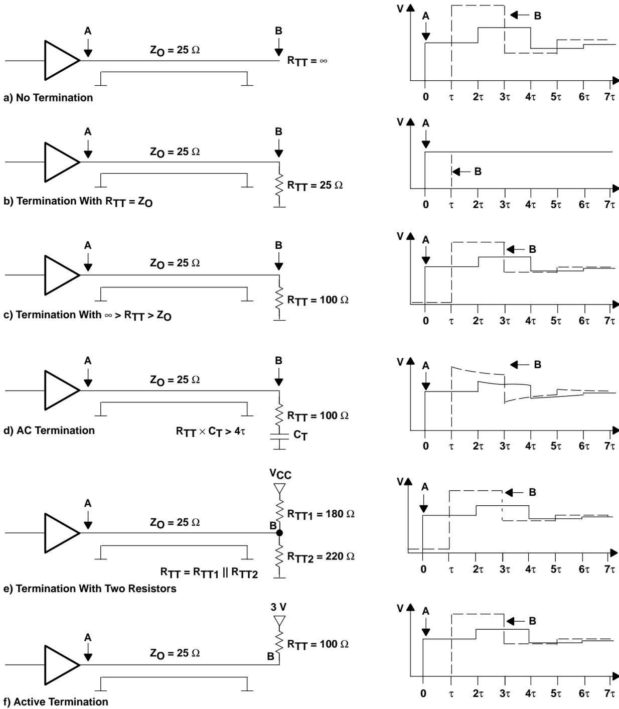
Figure 8. Termination Methods With TTL and CMOS Circuits
