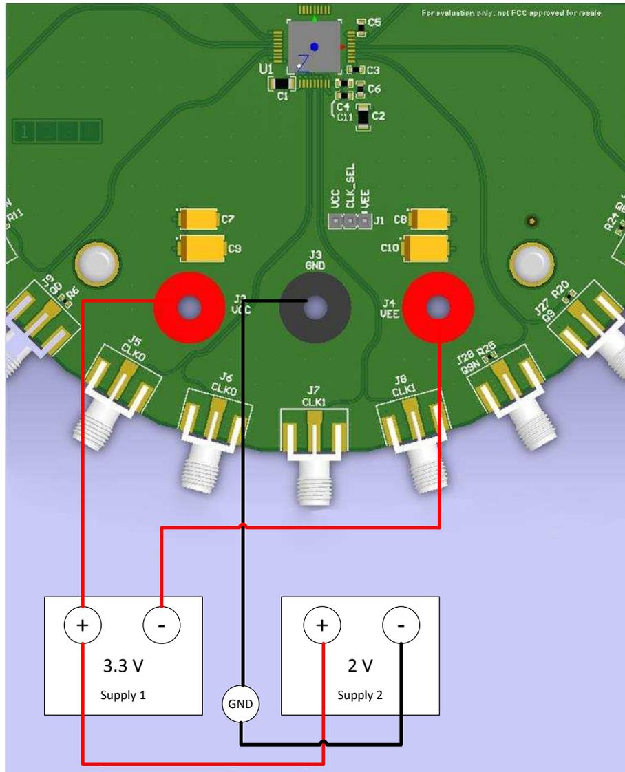
**Figure 2. Power Supply Connections**
