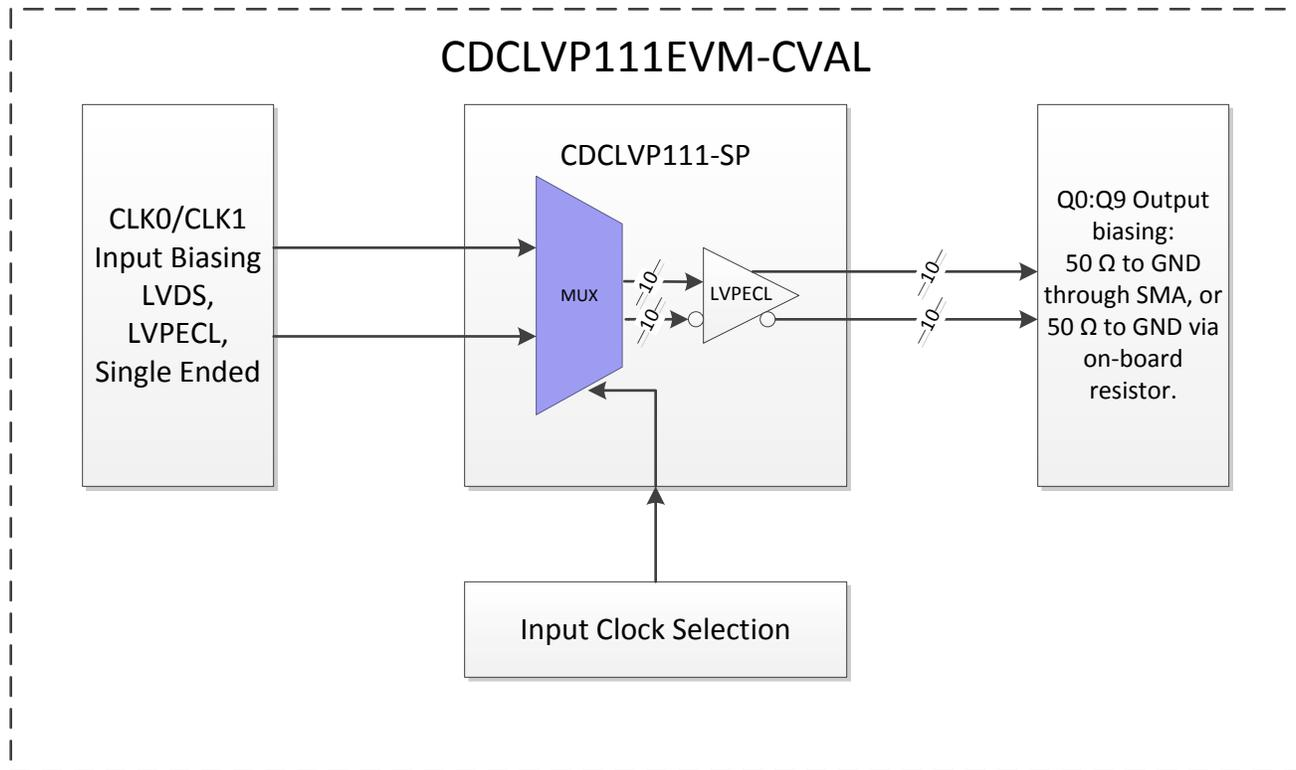
Figure 1. CDCLVP111-SP EVM Block Diagram
