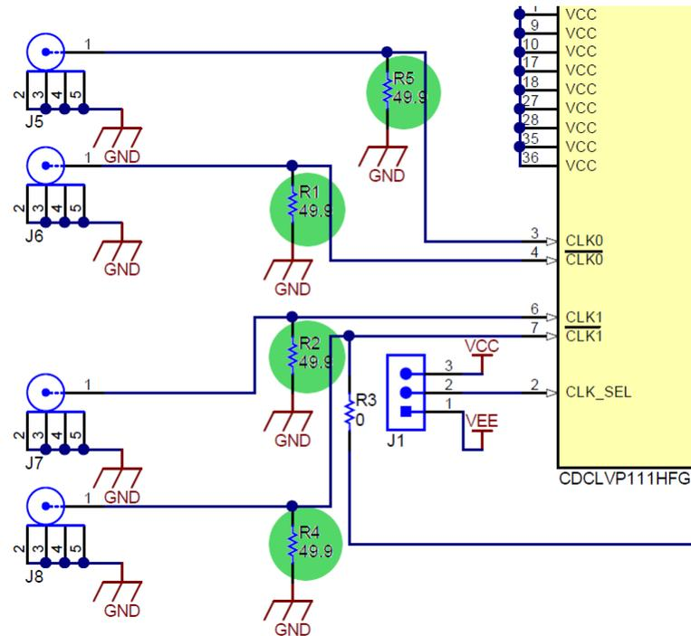
Figure 3. Input Biasing Schematic
