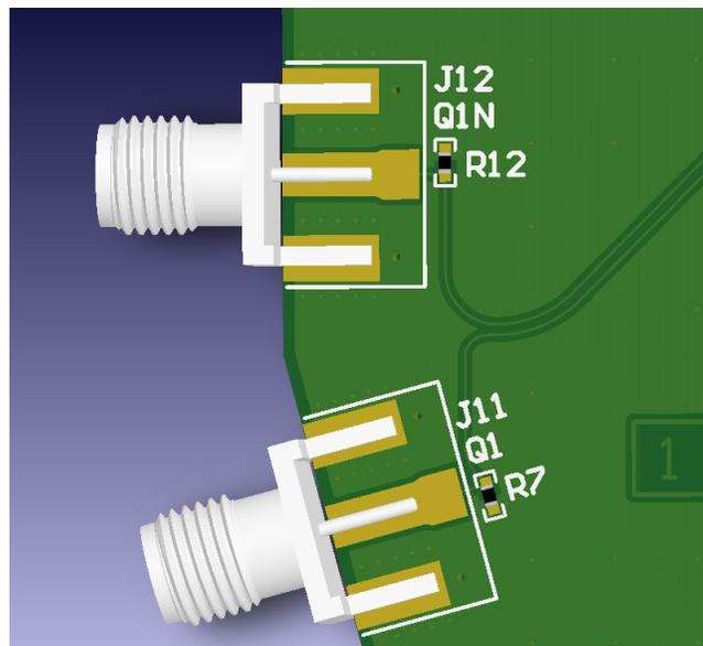
Figure 6. On Board Optional Output Termination
