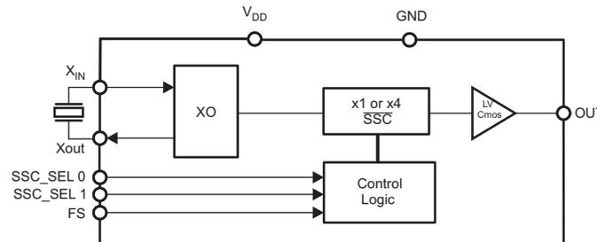
**Figure 3. Functional Block Diagram of the CDCS502**
