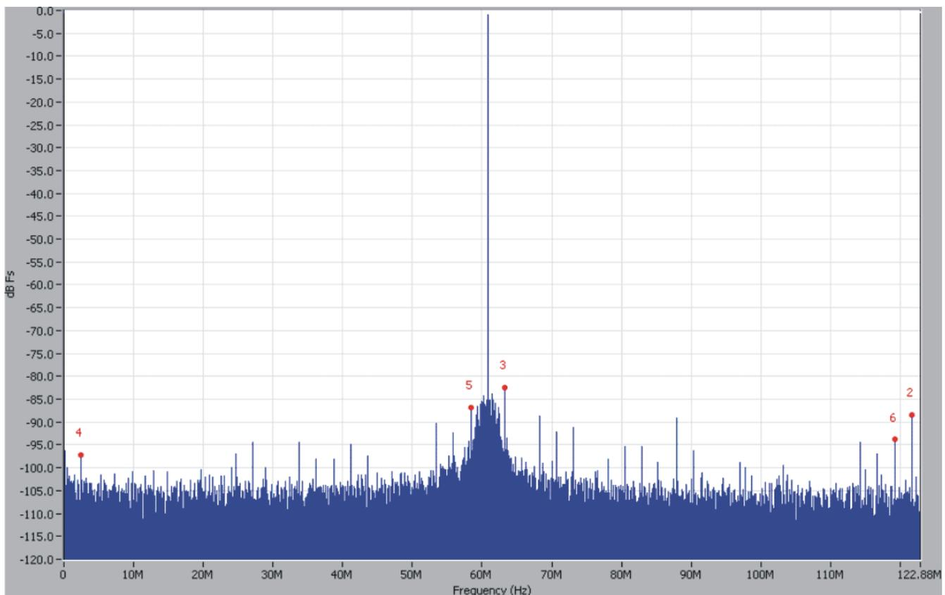
Figure 17. Spectral Performance with the CDCE62005-BPF-Transformer at 170-MHz IF Input
