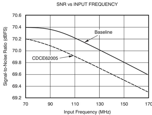
Figure 16. SNR Performance vs IF Input Frequency
