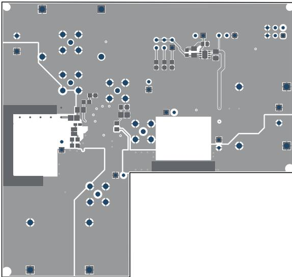
**Figure 3-8. Bottom Layer Routing**
