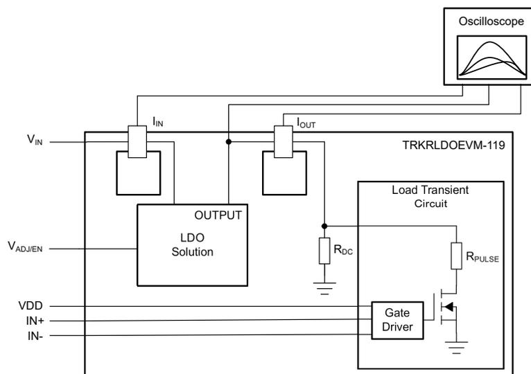
Figure 1-1. TRKRLDOEVM-119 Functional Block Diagram
