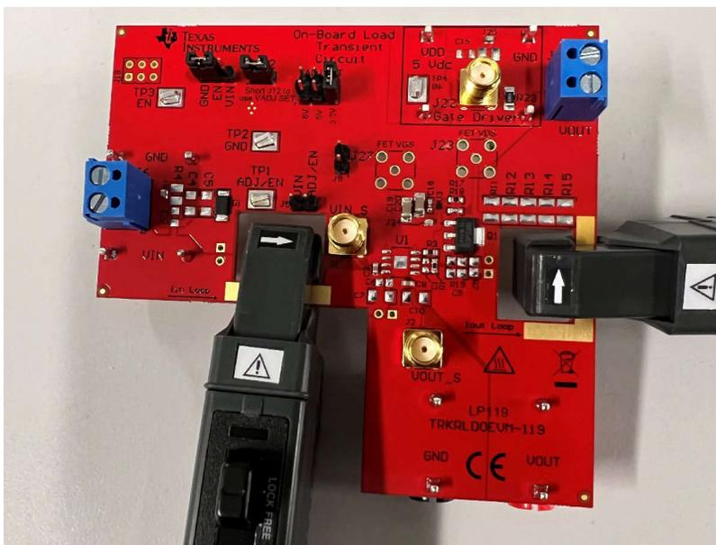
**Figure 2-1. TRKRLDOEVM-119 With Current Probes Attached**
