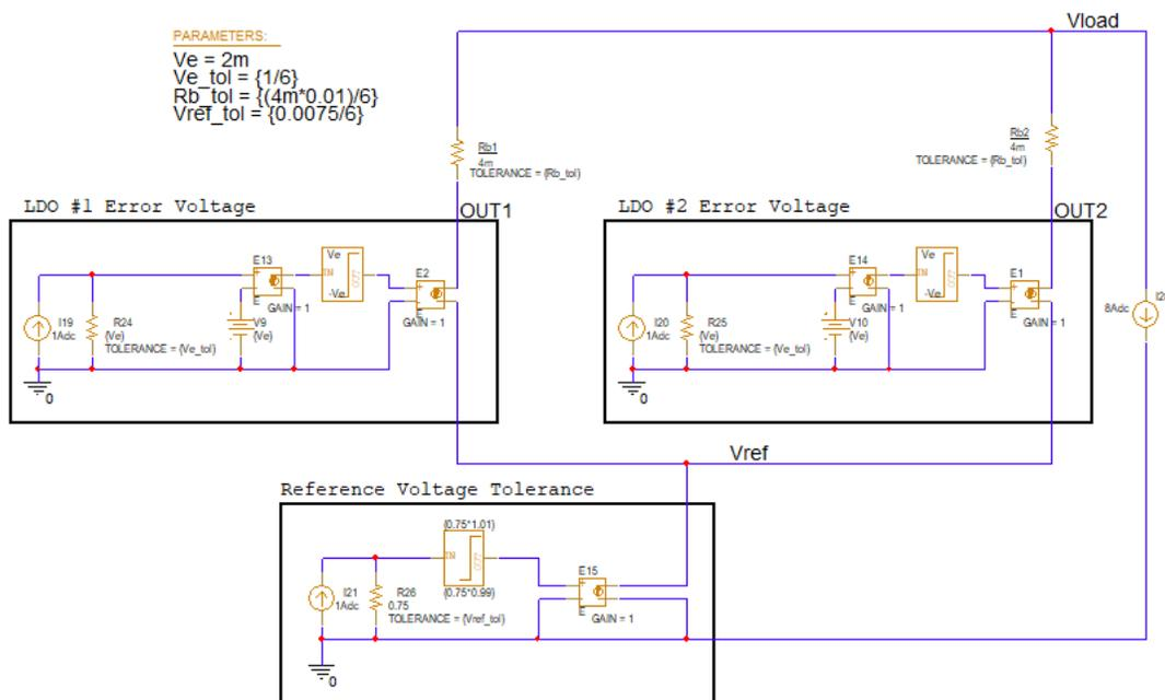
Figure 3-3. Modified PSpice Schematic to Simulate the  $I_{OUTn}$  Distribution of Two Parallel LDOs
