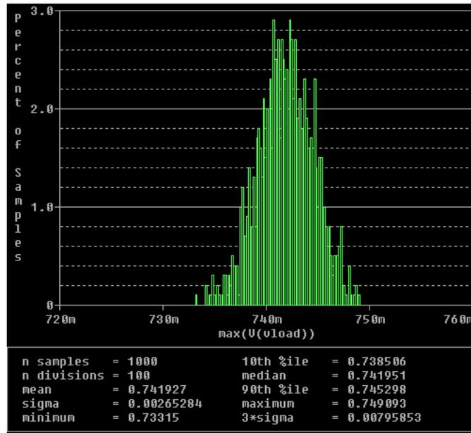
**Figure 3-7.  $V_{LOAD}$  Simulation Results**
