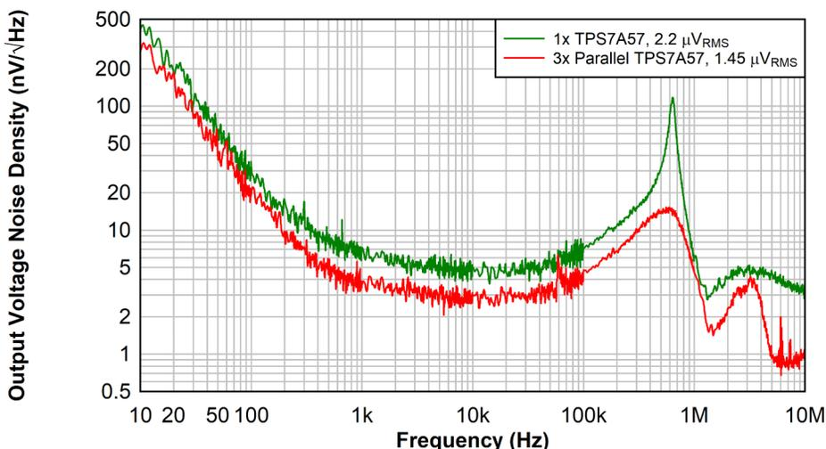
**Figure 2-1. Output Voltage Noise Density vs. Frequency**
