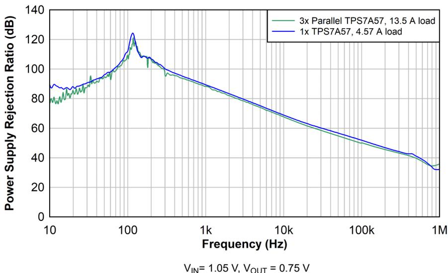
**Figure 2-2. PSRR vs. Frequency and  $I_{OUT}$  for 3x Parallel TPS7A57 and 1x Single TPS7A57**
