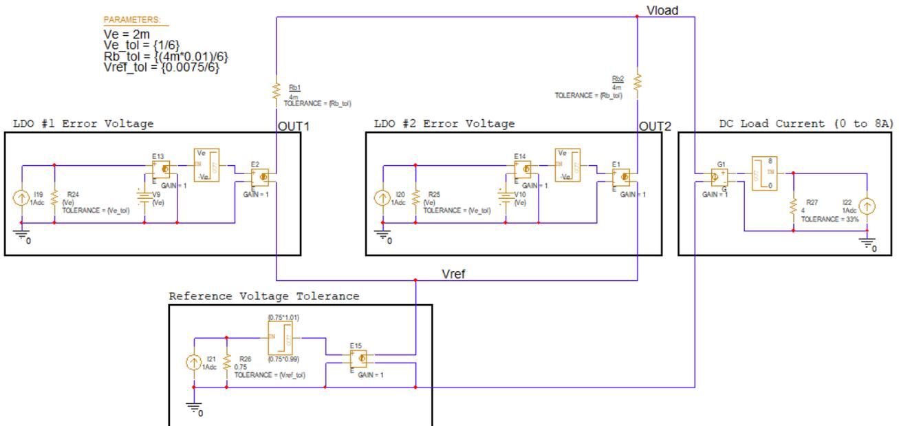
Figure 3-6. Modified PSpice Schematic to Simulate the  $V_{LOAD}$  Distribution of Two Parallel LDOs
