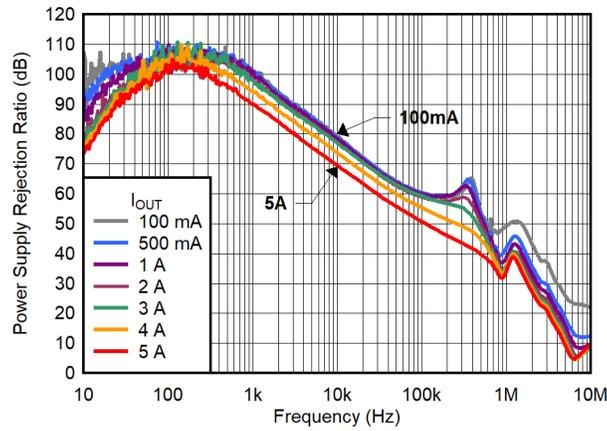
**Figure 4-4. TPS7A57 PSRR vs Frequency and  $I_{OUT}$  for CP Enabled, No Bias**
