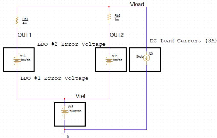
Figure 3-2. Spice Simulation Schematic of Two Parallel LDOs
