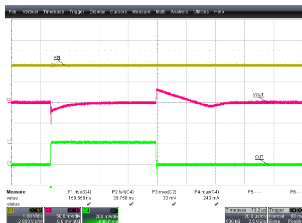
Figure 3-12. Current Probe Measurement with Shortened Cabling
