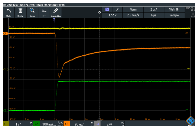
Figure 3-5. TLV773 Load Transient with SMA Connection
