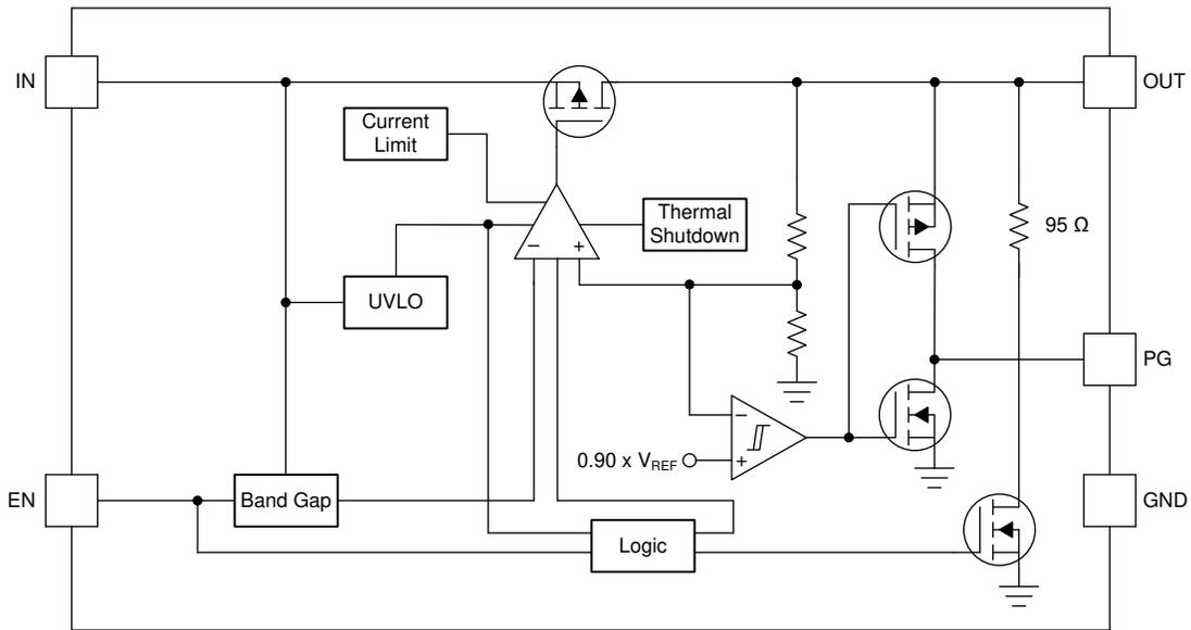
**Figure 1-4. Fixed Voltage Version With Push-Pull Power-Good**
