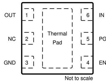
**Figure 4-2. Pin Diagram Fixed TPS745-Q1 DRV Package**
