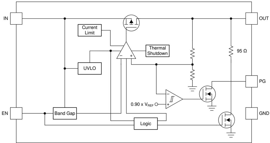
**Figure 1-3. Fixed Voltage Version With Open-Drain Power-Good**
