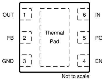
**Figure 4-1. Pin Diagram Adjustable TPS745-Q1 DRV Package**
