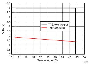
Figure 4. Using TMP20 and TPS3701 to detect for under- and over-temperature
