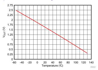
Figure 3. V<sub>out</sub> vs. Temperature for TMP20 over the entire temperature range
