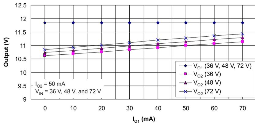
Figure 5. Regulation with IO<sub>UT2</sub> = 50 mA
