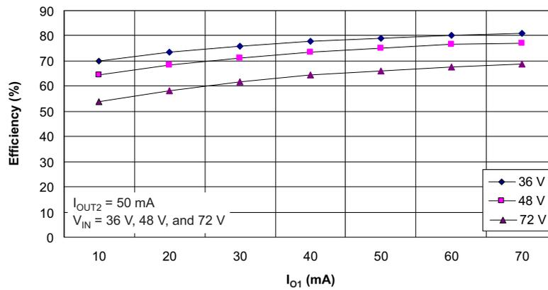
Figure 3. Efficiency with IOUT2 = 50 mA
