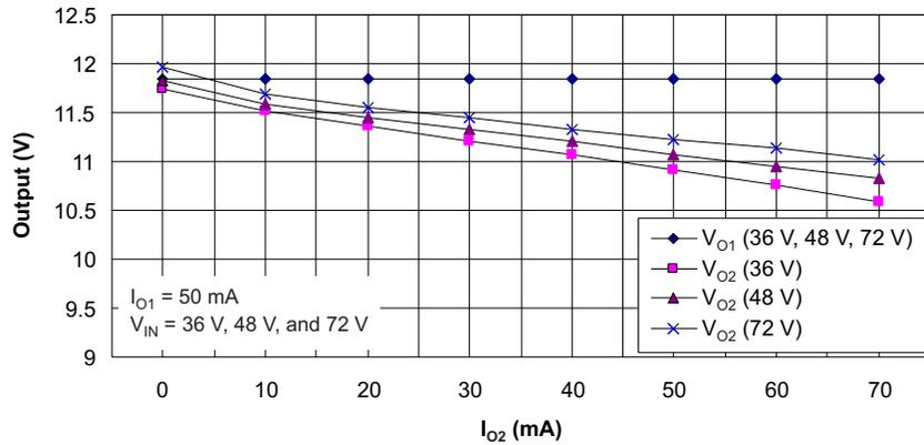
Figure 4. Regulation with IO<sub>UT1</sub> = 50 mA
