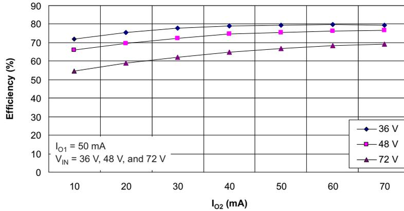
Figure 2. Efficiency with IOUT1 = 50 mA
