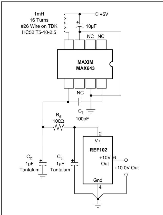
FIGURE 3. +10.0V Reference Using REF102 Can Operate on Single +5V Power Supply.
