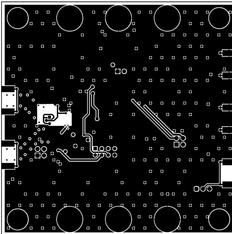
**Figure 3-7. Bottom Layer PCB Layout**
