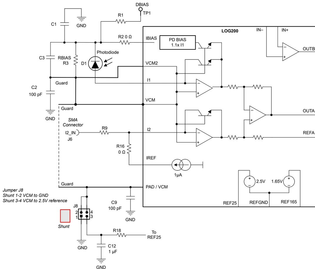
**Figure 2-3. LOG200EVM Photodiode Connections**
