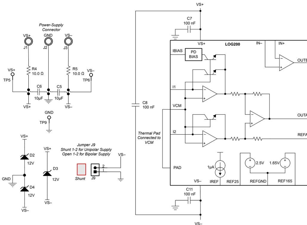
**Figure 2-1. LOG200EVM Voltage Supply Connections**
