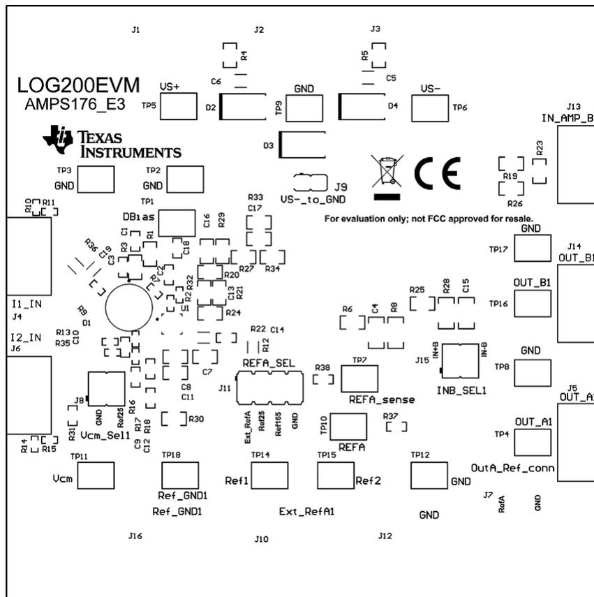
Figure 3-3. Top Overlay PCB Layout
