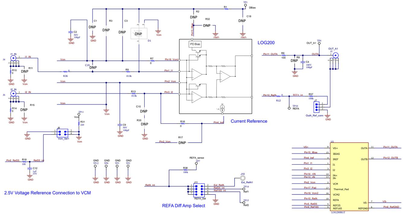
Rev E3: Modified REF25 connection to VCM, through REF25 filter: R18=100Ohm, C12=1uF. Modified Capacitors values C2, C9 from 1000pF to 100pF. Modified REF165 bypass capacitor C14 from 330pF to 100pF. Added C19, R36, R37, R38, TP7 for flexibility.
