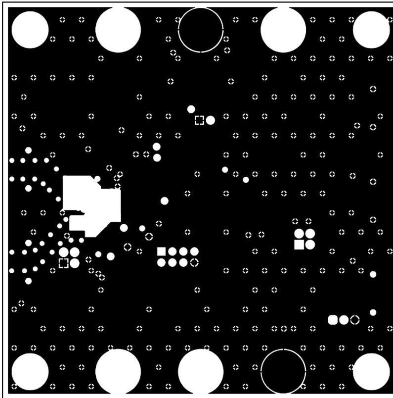
**Figure 3-6. Mid Layer 2 PCB Layout**
