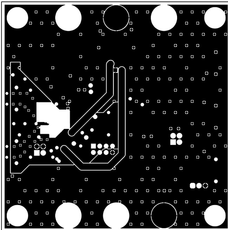
**Figure 3-5. Mid Layer 1 PCB Layout**
