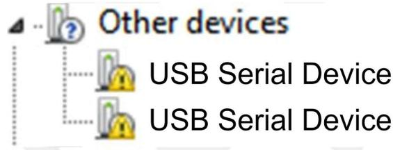
Figure 5-1. OPTEVM on Microsoft® Windows® 7 With Drivers not Installed
