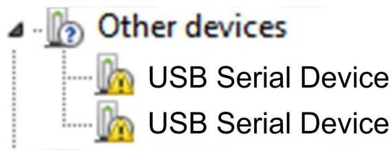
Figure 5-1. OPT4001YMNEVM on Microsoft® Windows® 7 With Drivers not Installed
