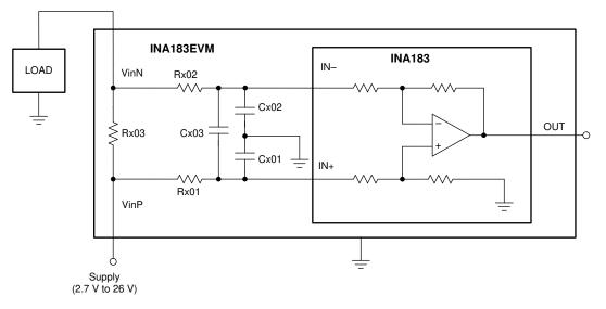
Figure 3-1. Measurement With Shunt
