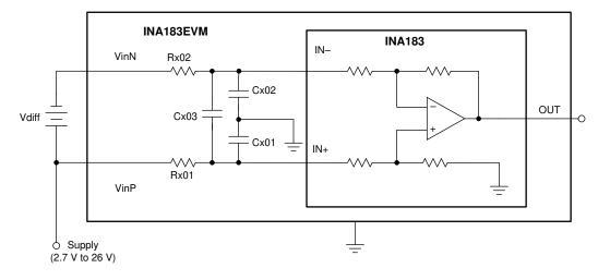
Figure 3-2. Measurement Without Shunt
