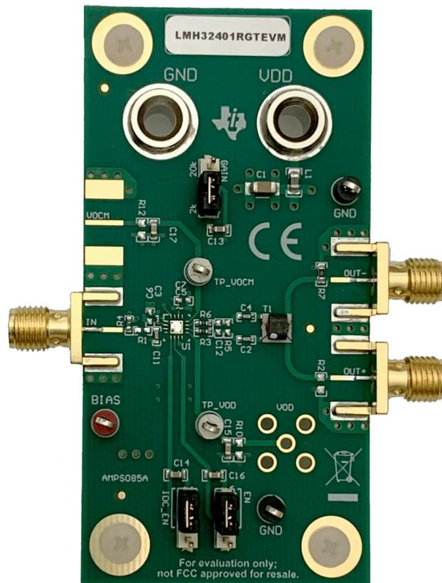
This user's guide describes the characteristics, operation, and use of the LMH32401RGTEVM. This evaluation module (EVM) is an evaluation and development kit for evaluating the LMH32401IRGT device, a programmable-gain, single-ended input to differential output transimpedance amplifier for light detection and ranging (LIDAR) applications and laser distance measurement systems. A complete circuit description as well as schematic diagram and bill of materials are included in this document.
