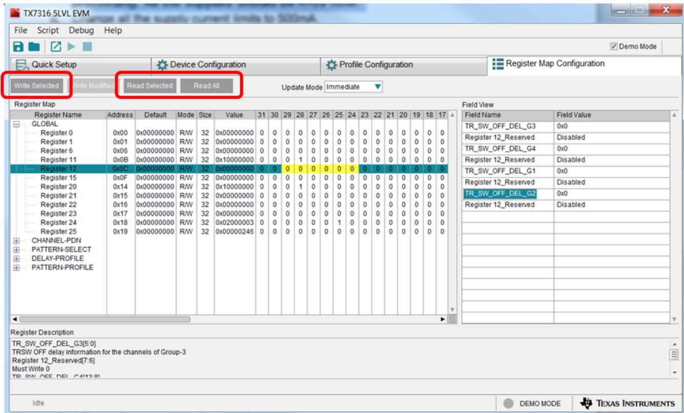
Figure 37. Register Map Configuration – Update Mode (Immediate)
