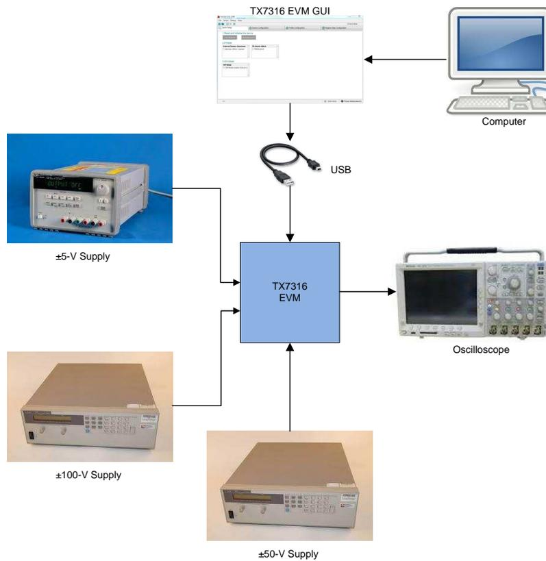
Figure 3. On-chip Beamforming Setup
