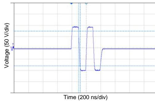
Frequency = 5 MHz; Peak-to-Peak = 196.5 mV, Rise Time = 20.8 ns; Fall Time = 21 ns
