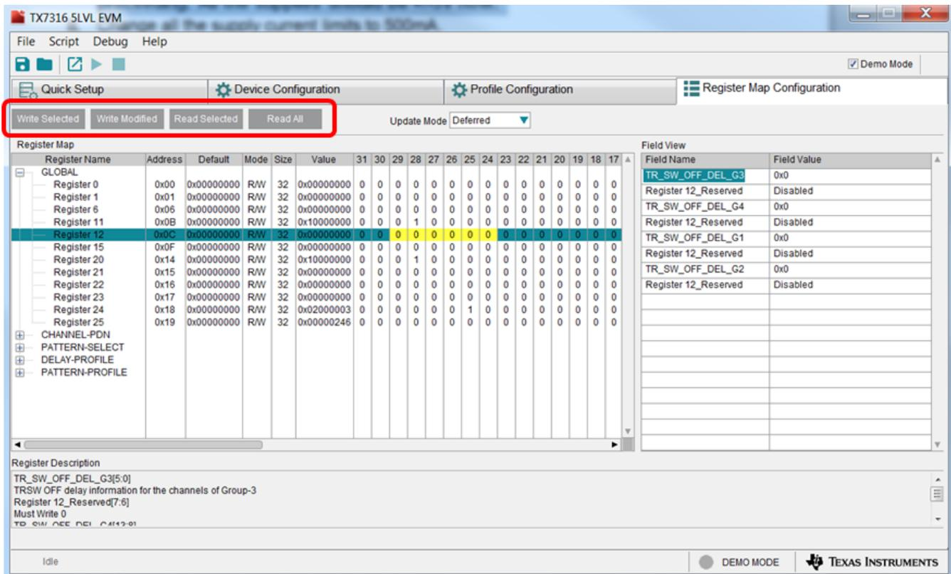
Figure 38. Register Map Configuration – Update Mode (Deferred)
