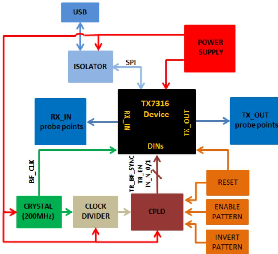
Figure 51. EVM Hardware Block Diagram
