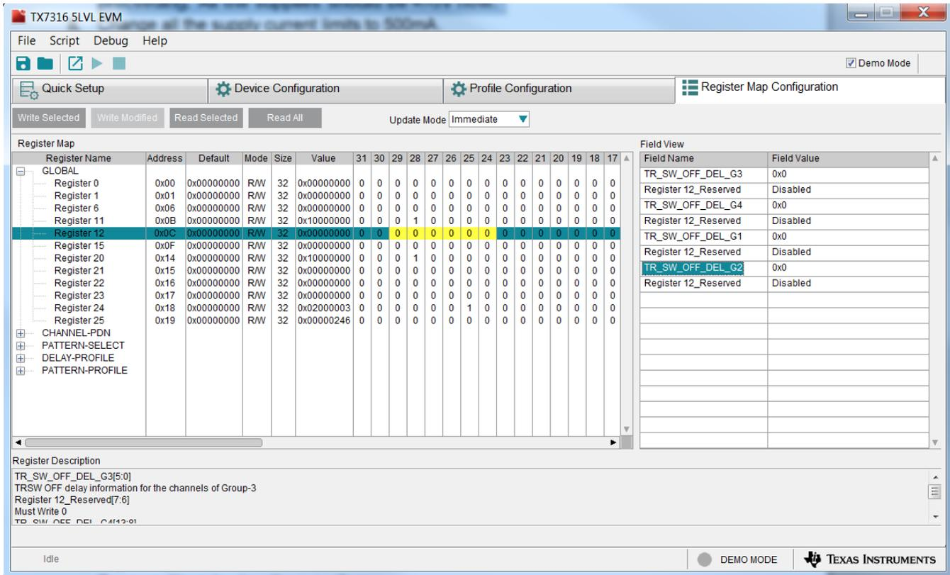
Figure 35. Register Map Configuration – Field View
