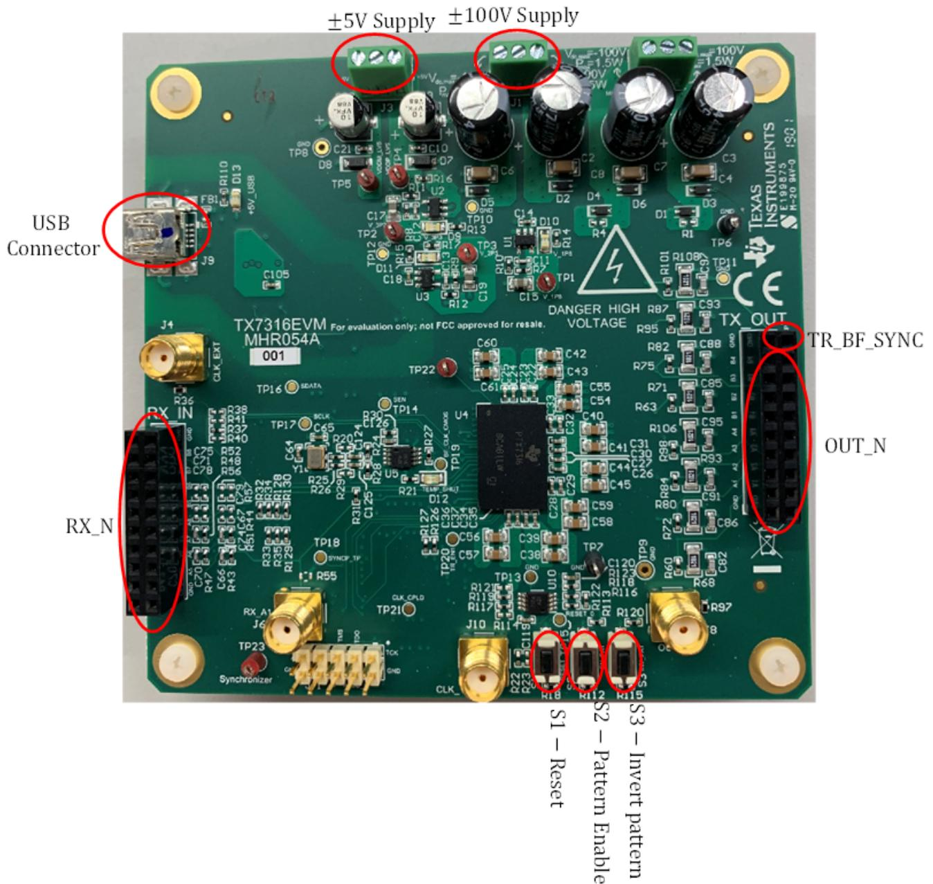
Figure 40. Connectors and Switches of the EVM
