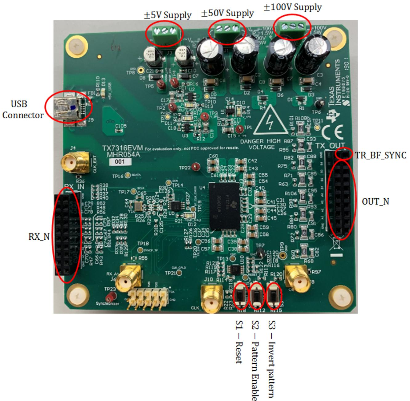
Figure 4. Connectors and Switches of the EVM
