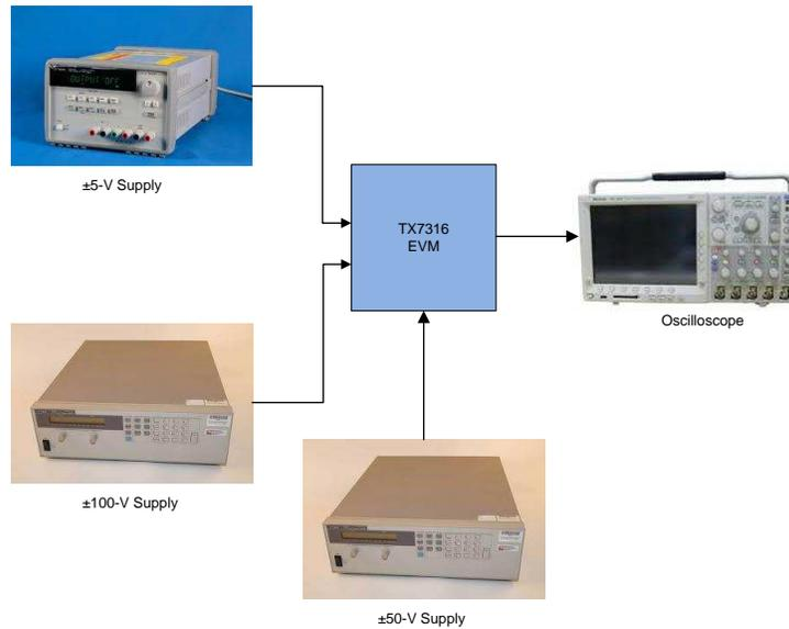
Figure 2. Off-chip Beamforming Setup
