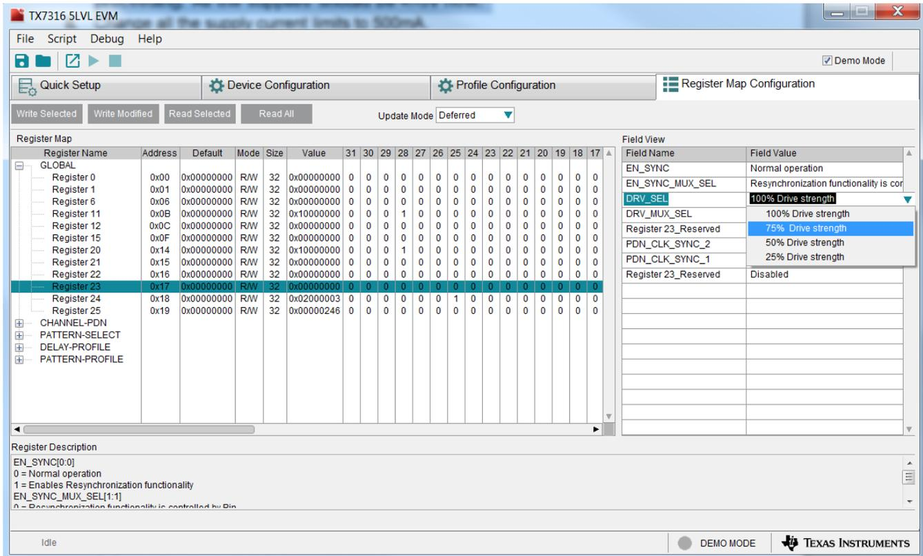
Figure 39. Register Map Configuration – Changing Register Value
